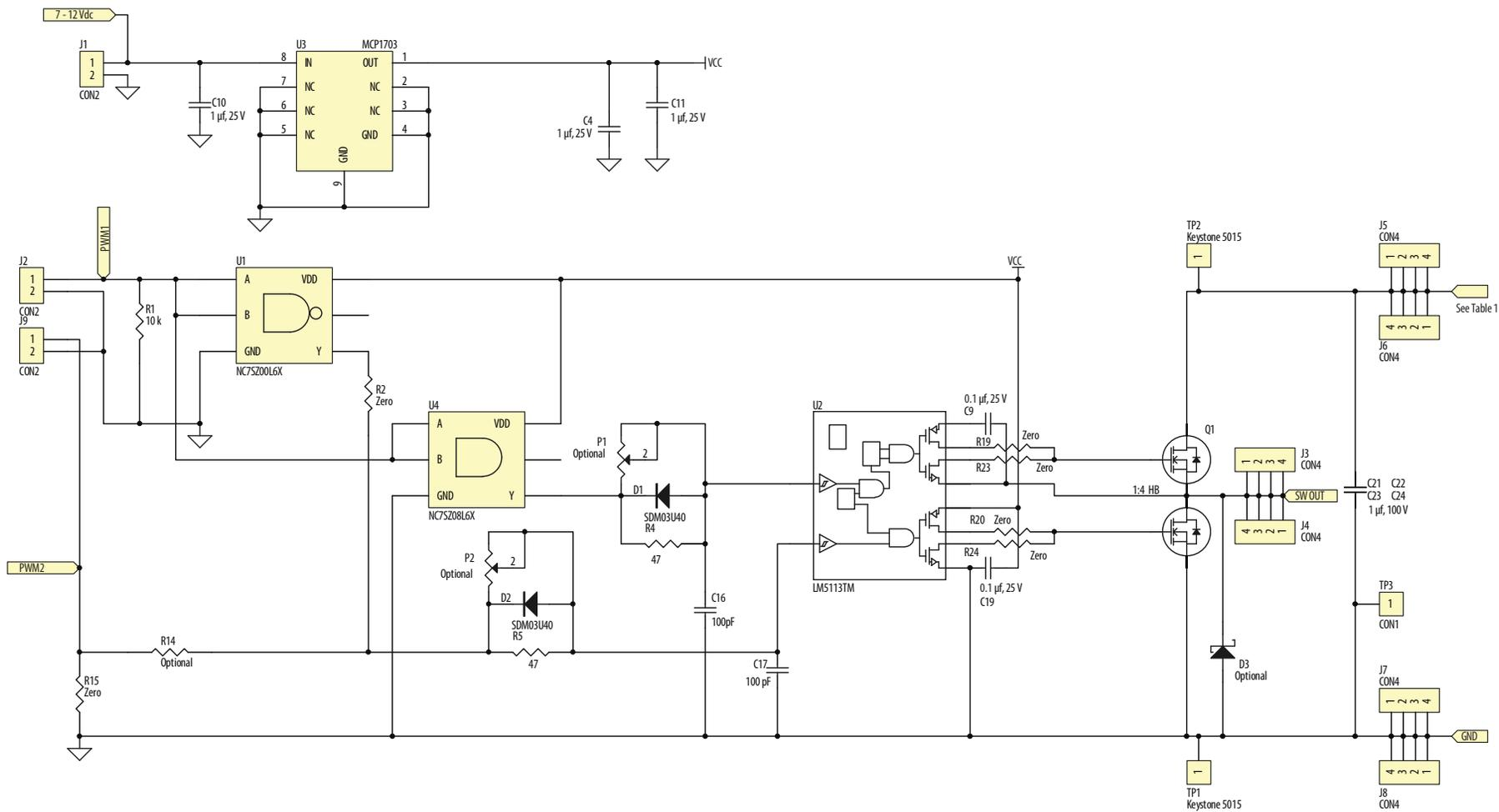
Figure 4: EPC9041 Development Board Schematic
