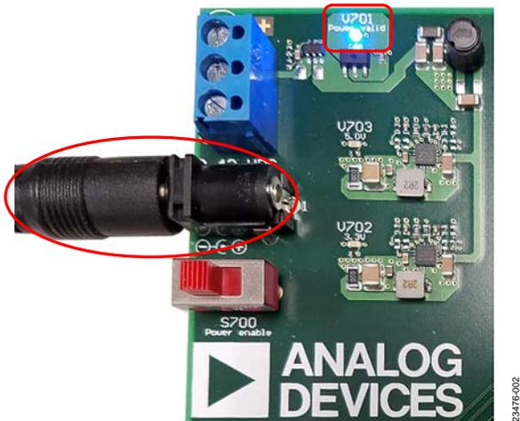
Figure 2. Power Cable Connection and Power Valid LED
