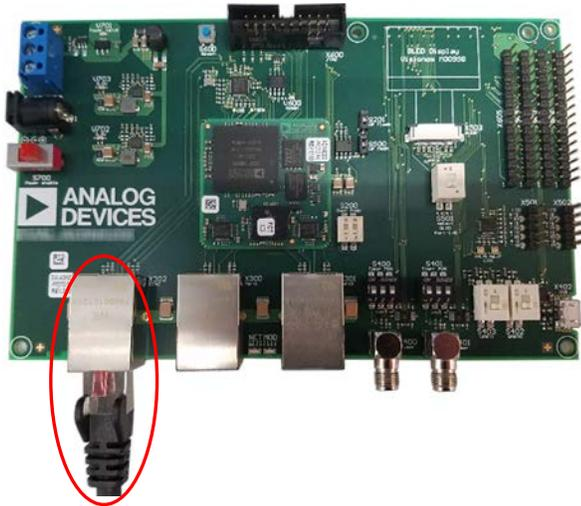
Figure 5. Ethernet Cable Connection
