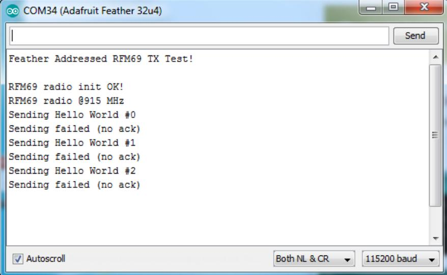
A screenshot of a serial console window titled "COM34 (Adafruit Feather 32u4)". The window contains the following text: "Feather Addressed RFM69 TX Test!", "RFM69 radio init OK!", "RFM69 radio @915 MHz", "Sending Hello World #0", "Sending failed (no ack)", "Sending Hello World #1", "Sending failed (no ack)", "Sending Hello World #2", "Sending failed (no ack)". At the bottom of the window, there are controls for "Autoscroll" (checked), "Both NL & CR" (dropdown), and "115200 baud" (dropdown).
