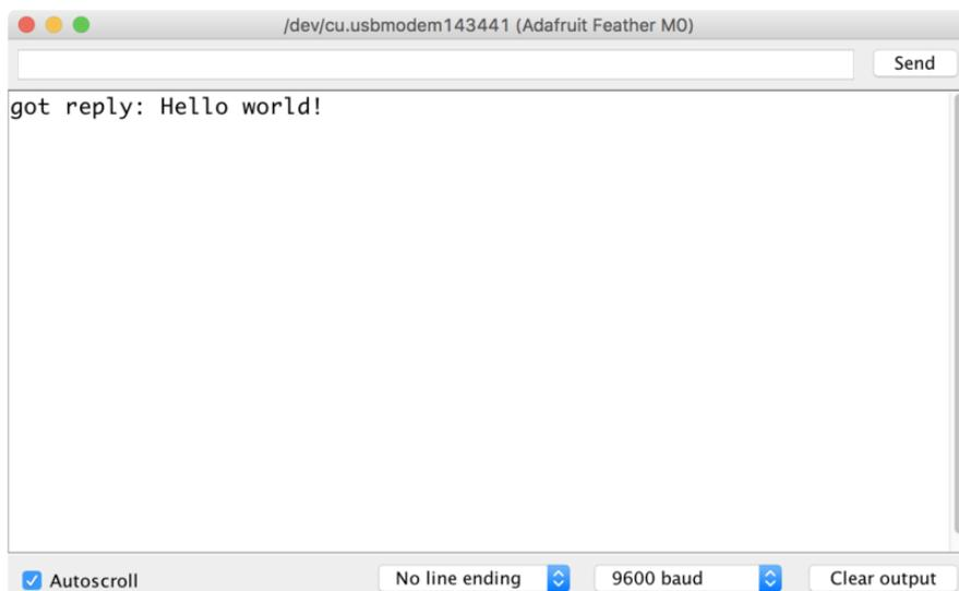
To receive a message simply call the `receive` function. This function will wait for half a second for any packet to be received. If a packet is found it will be returned as a byte string (remember packets are at most 252 bytes long), or if no packet was found a result of `None` is returned.
