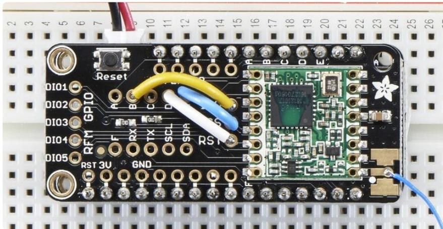
Because each Feather uses a different processor, there is some light wiring that needs to be done to configure the radio pins. In particular, an interrupt-capable pin is required for IRQ but there is no one interrupt pin that is consistent across all Feather boards!
