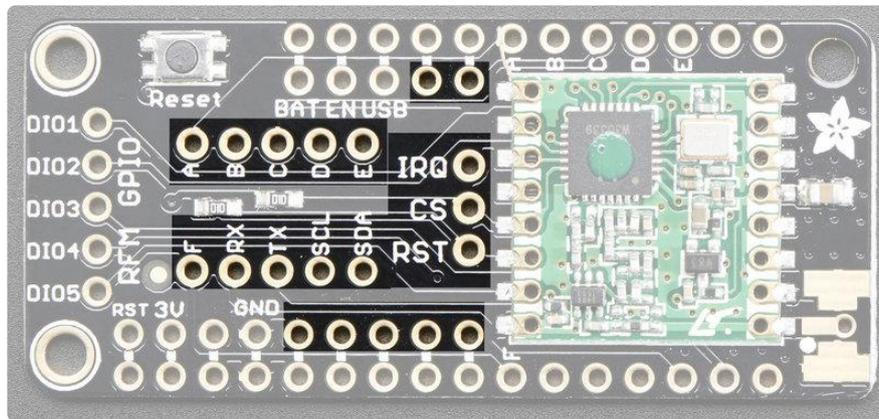
Three wires from IRQ, CS and RST will be soldered to three of these other points. Exactly which pins to connect are shown on the next page (it varies among Feather boards), this is merely to illustrate how the short soldered wires might look when installed:
