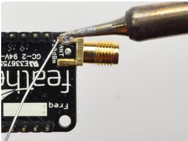
Solder all 5 connections (4 ground/mechanical and 1 signal)
