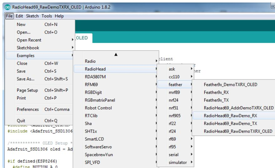
Before uploading, check for the `#define RF69_FREQ` line and edit if necessary to match the frequency of the radio hardware you're using.
