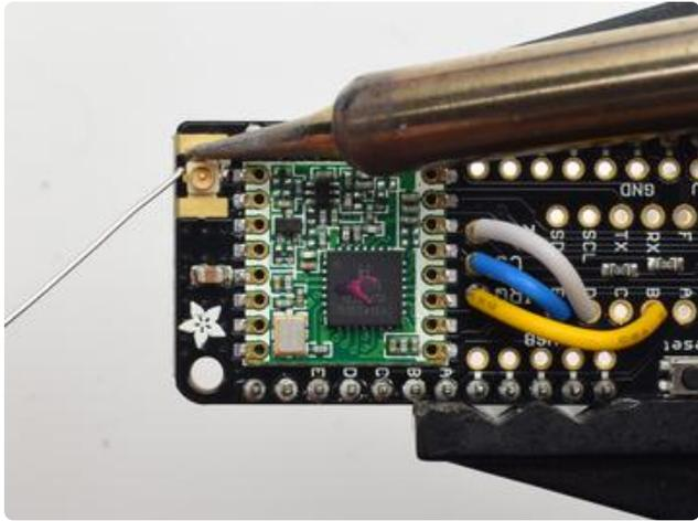
Solder in the two side pads, they are used for signal and mechanical connectivity so make sure there's plenty of solder
