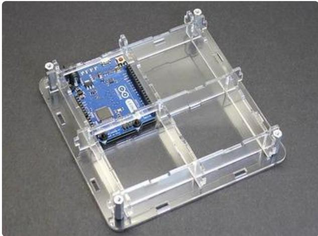
The horizontal braces now slot into notches on the verticals. Each of these is a different shape. The thinnest one is designed to clear the Arduino's power jack. The slightly thicker (but still pretty thin) brace goes down the middle, while the full-thickness one is at the bottom.
