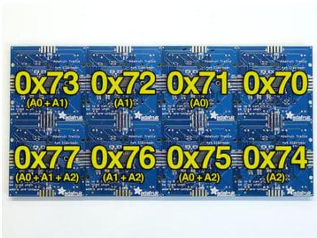
Here’s the address map for the HELLA UNTZtrument.
