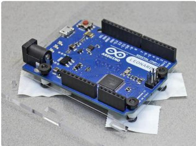
Install the Arduino board with the mounting holes over these three screws (there's a fourth hole, but we're not using it here).
