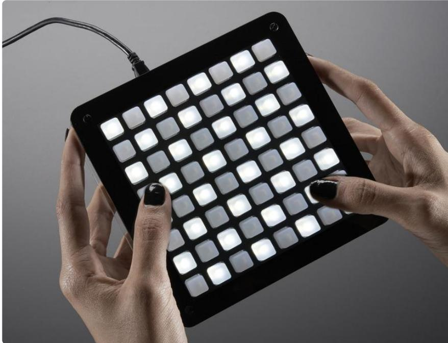
Build and customize your very own open-source button grid controller with UNTZtrument! This DIY kit comes with delicious translucent button pads, driver boards, diffused white LEDs and a custom laser cut enclosure. The result is a sturdy and elegant but also super-hackable controller for music, video...or something else???
