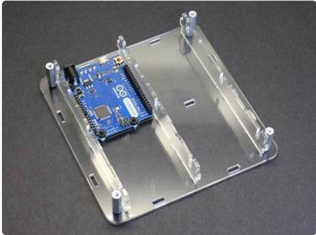
The vertical braces (which run parallel to the Arduino's longer axis) all look similar, but notice the "nubs" on the bottom are different: one, two, one. These fit into corresponding slots on the base. (On the HELLA UNTZtrument, there are five vertical braces — again, they're keyed to only fit specific positions).
