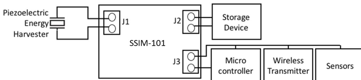
Figure 4. Example 1: Wireless sensor node with SSIM-101
