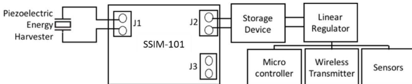
Figure 5. Example 2: Wireless sensor node with SSIM-101
