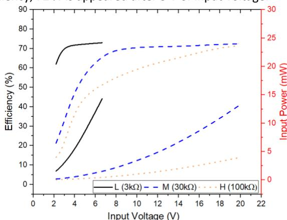
Figure 2. Efficiency vs. Input Voltage / Power
