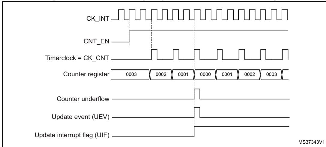
**Figure 253. Counter timing diagram, internal clock divided by 4, TIMx\_ARR=0x36**
