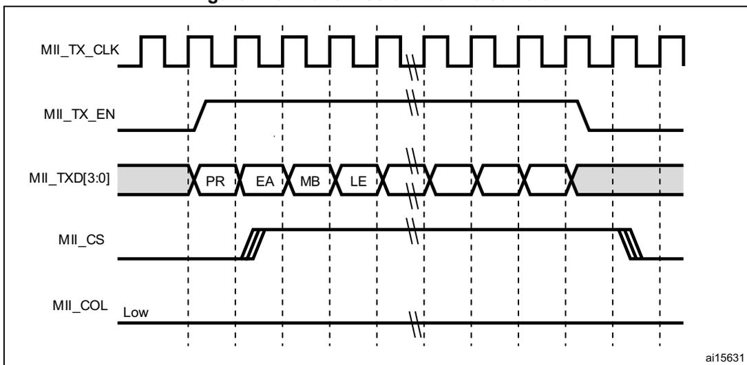
Figure 477. Transmission with collision
