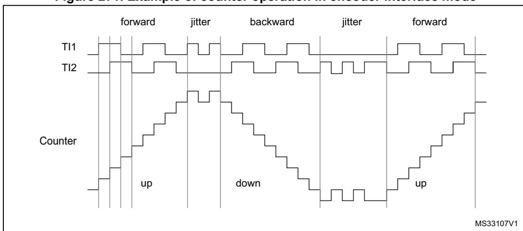
Figure 272 gives an example of counter behavior when TI1FP1 polarity is inverted (same configuration as above except CC1P=1).
