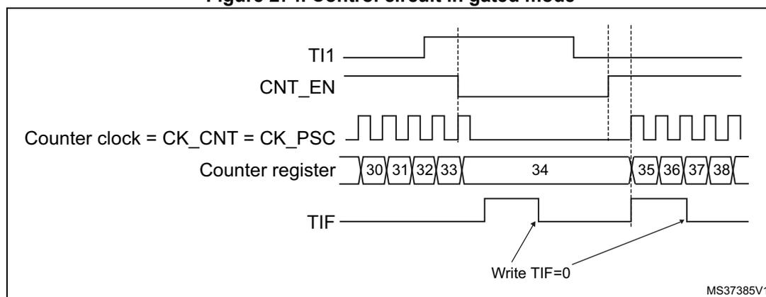
1. The configuration "CCxP=CCxNP=1" (detection of both rising and falling edges) does not have any effect in gated mode because gated mode acts on a level and not on an edge.
