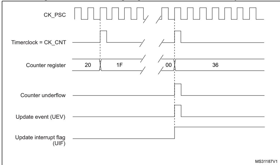
**Figure 202. Counter timing diagram, update event when repetition counter is not used**
