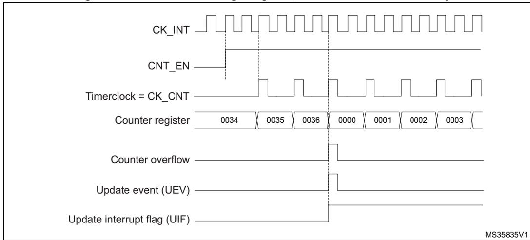
**Figure 242. Counter timing diagram, internal clock divided by 4**
