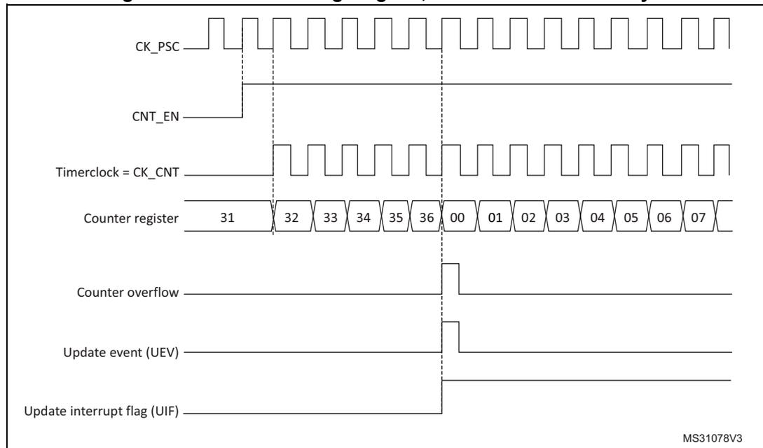
**Figure 288. Counter timing diagram, internal clock divided by 2**
