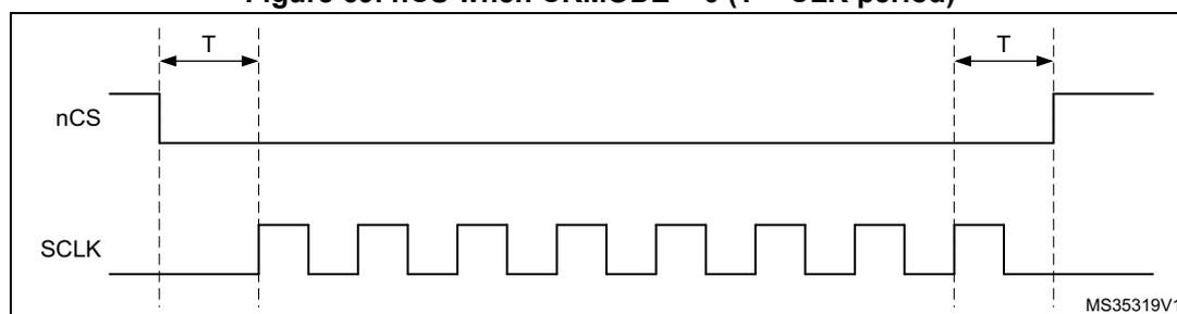
When CKMODE=1 (“mode3”, where CLK goes high when no operation is in progress) and DDRM=0 (SDR mode), nCS still falls one CLK cycle before an operation first rising CLK edge, and nCS rises one CLK cycle after the operation final rising CLK edge, as shown in [Figure 70](#).
