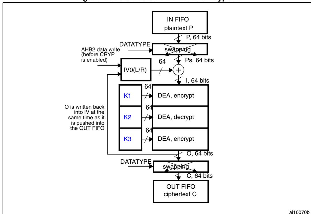
K: key; C: cipher text; I: input block; O: output block; Ps: plain text before swapping (when decoding) or after swapping (when encoding); P: plain text; IV: initialization vectors.
