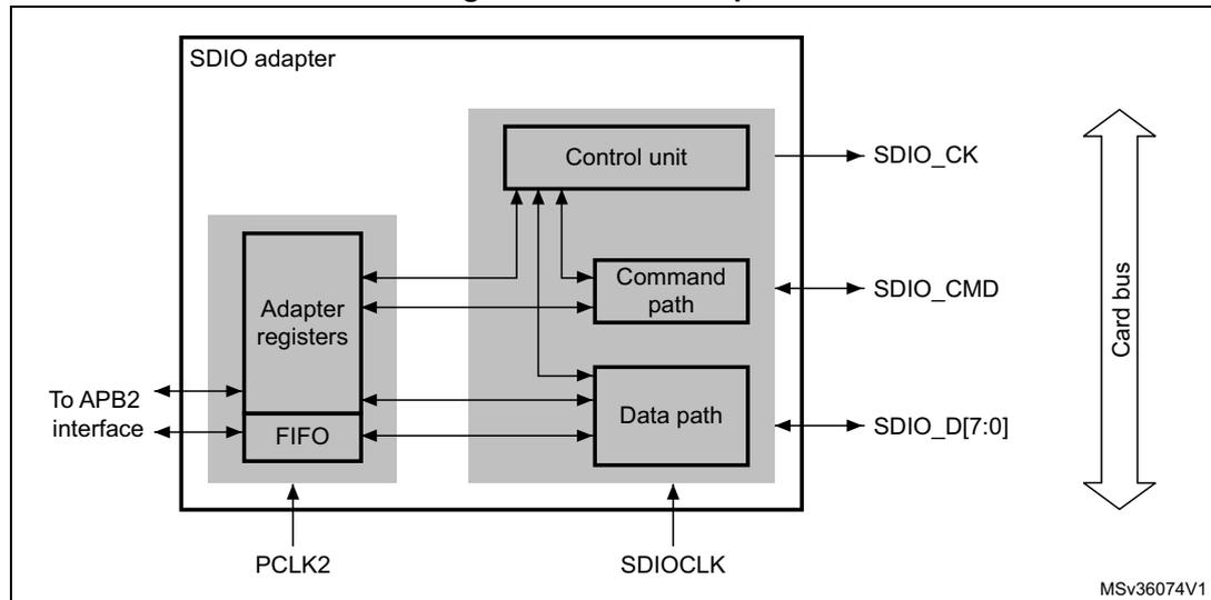
The SDIO adapter is a multimedia/secure digital memory card bus master that provides an interface to a multimedia card stack or to a secure digital memory card. It consists of five subunits:
