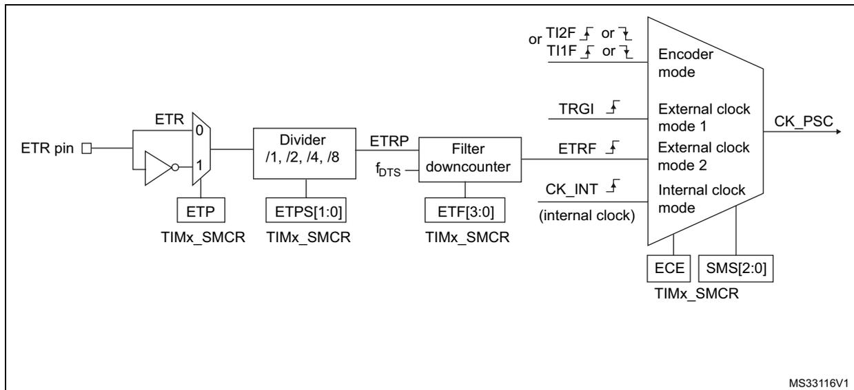
For example, to configure the upcounter to count each 2 rising edges on ETR, use the following procedure:
