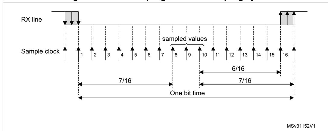
Figure 333. Data sampling when oversampling by 8
