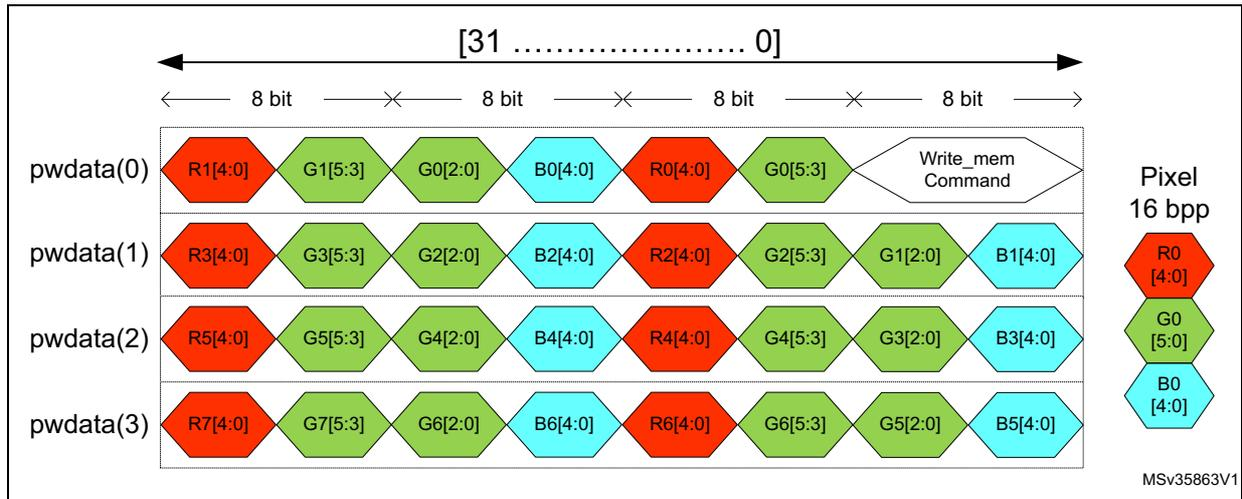
Figure 128. 12 bpp APB pixel to byte organization
