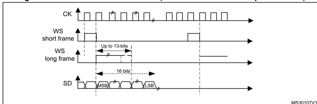
*Note:* For both modes (master and slave) and for both synchronizations (short and long), the number of bits between two consecutive pieces of data (and so two synchronization signals) needs to be specified (DATLEN and CHLEN bits in the SPIx\_I2SCFGR register) even in slave mode.
