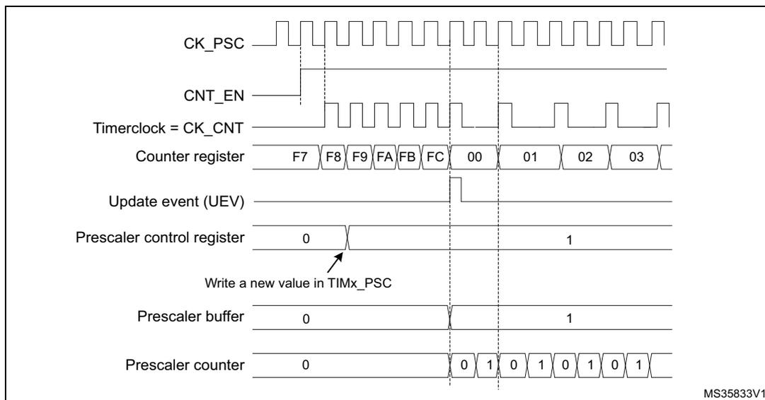
Figure 239. Counter timing diagram with prescaler division change from 1 to 4
