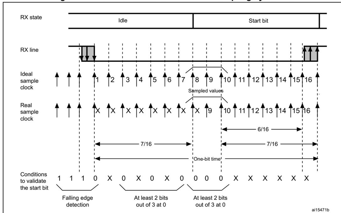
**Note:** *If the sequence is not complete, the start bit detection aborts and the receiver returns to the idle state (no flag is set) where it waits for a falling edge.*
