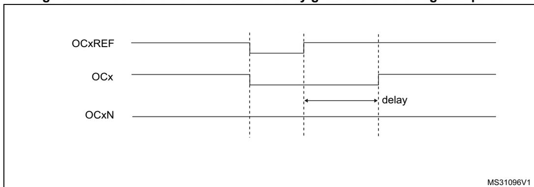
**Figure 225. Dead-time waveforms with delay greater than the positive pulse.**
