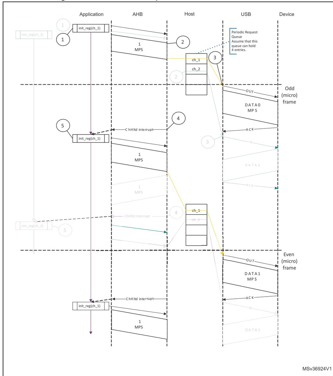
• **Interrupt IN transactions in DMA mode**
