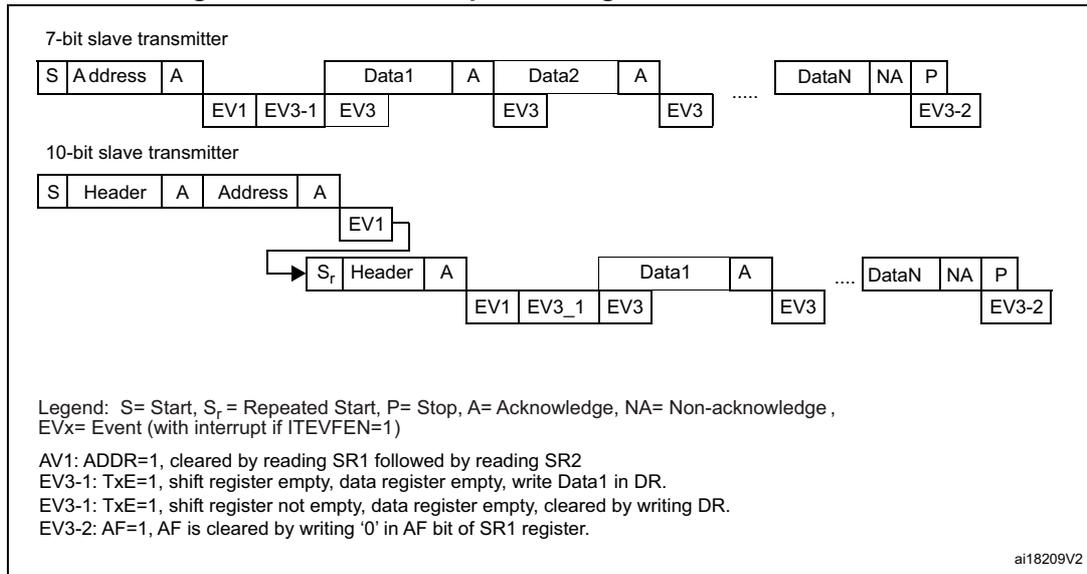
1. The EV1 and EV3\_1 events stretch SCL low until the end of the corresponding software sequence.
