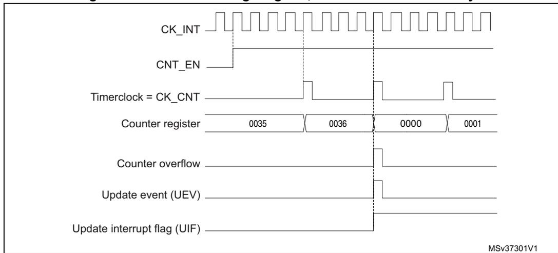
**Figure 312. Counter timing diagram, internal clock divided by N**
