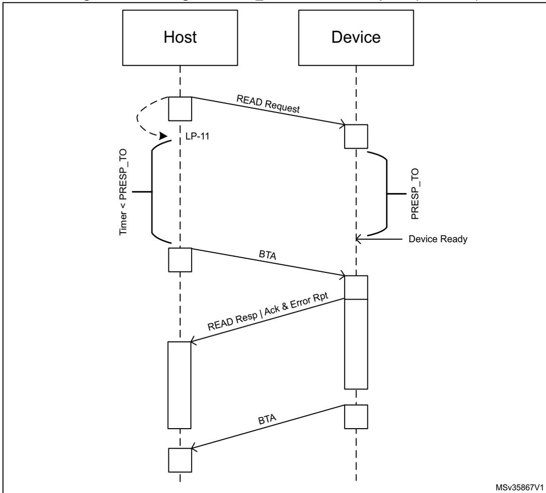
Figure 132. Timing of PRESP\_TO after a write request (HS or LP)
