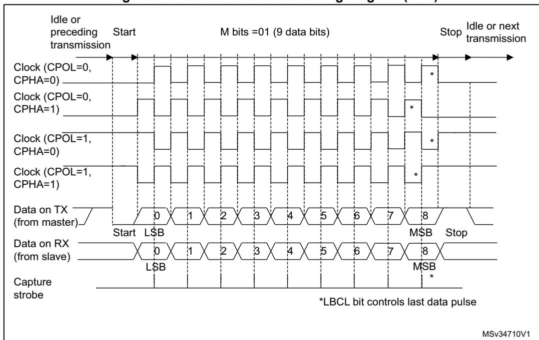
Figure 341. RX data setup/hold time
