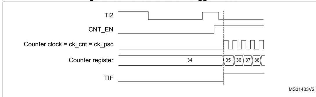
**Slave mode: external clock mode 2 + trigger mode**
