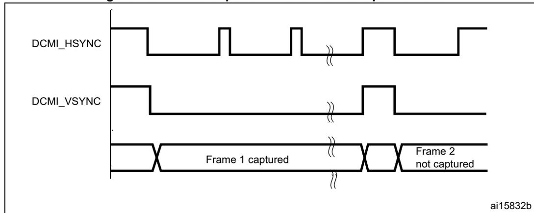
1. Here, the active state of DCMI\_HSYNC and DCMI\_VSYNC is 1.
