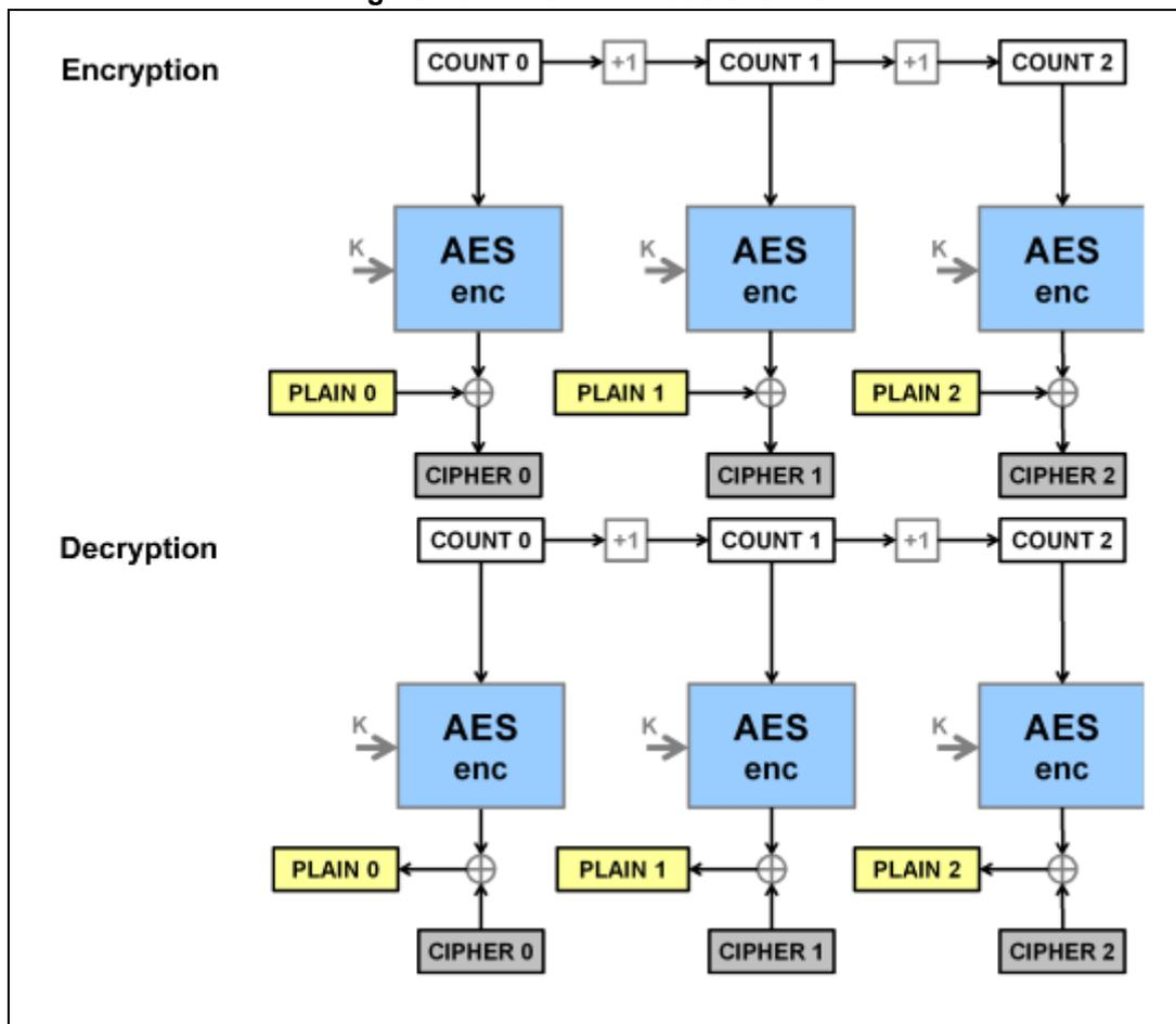
The CTR mode uses the AES core to generate a key stream; these keys are then XORed with the plaintext to obtain the ciphertext as specified in NIST *Special Publication 800-38A, Recommendation for Block Cipher Modes of Operation*.
