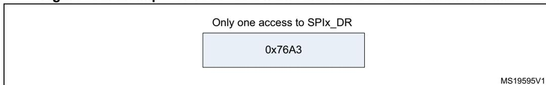
For transmission, each time an MSB is written to SPIx\_DR, the TXE flag is set and its interrupt, if allowed, is generated to load the SPIx\_DR register with the new value to send. This takes place even if 0x0000 have not yet been sent because it is done by hardware.
