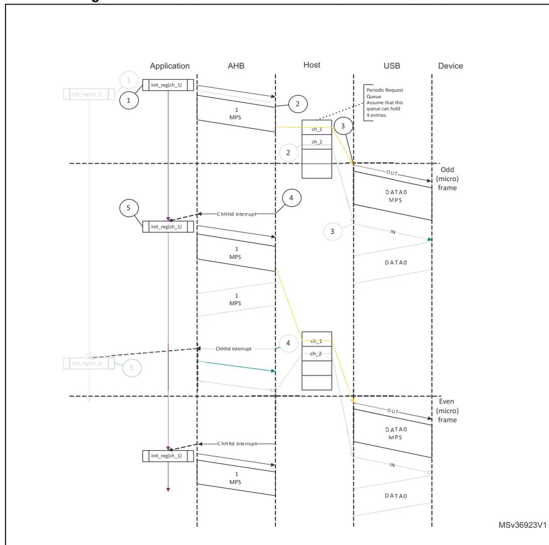
• **Isochronous IN transactions in DMA mode**
