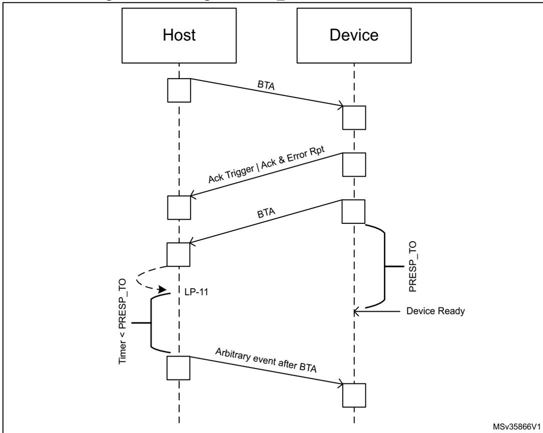
Figure 131. Timing of PRESP\_TO after a read request (HS or LP)
