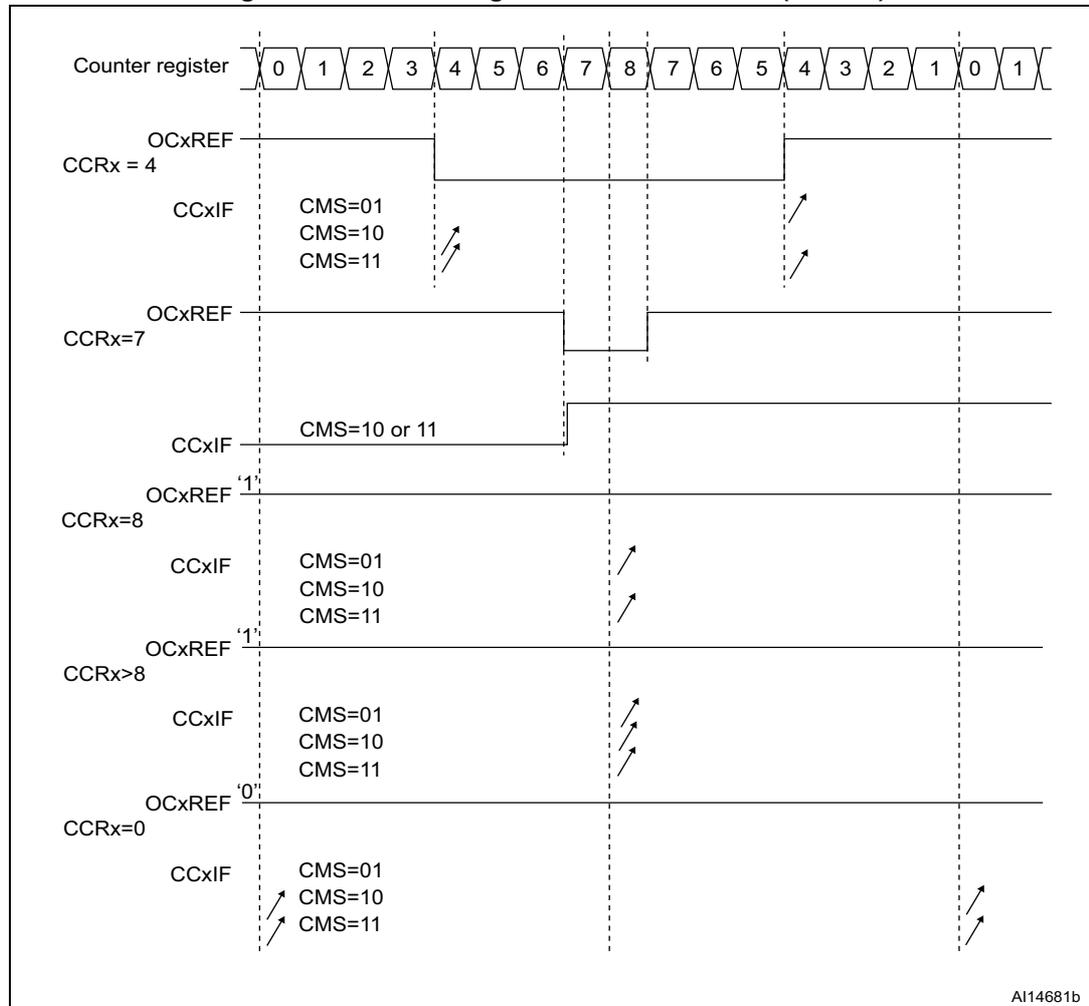
**Hints on using center-aligned mode:**
