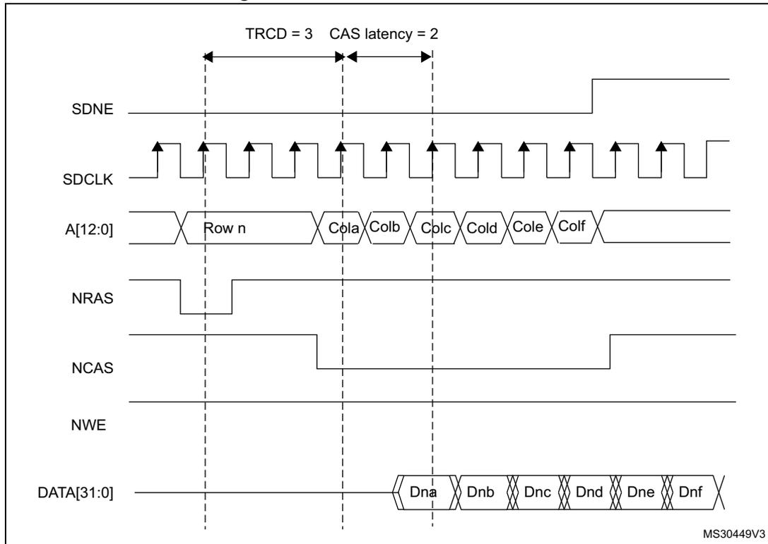
The FMC SDRAM controller features a Cacheable read FIFO (6 lines x 32 bits). It is used to store data read in advance during the CAS latency period and the RPIPE delay following the below formula. The RBURST bit must be set in the FMC\_SDCR1 register to anticipate the next read access.
