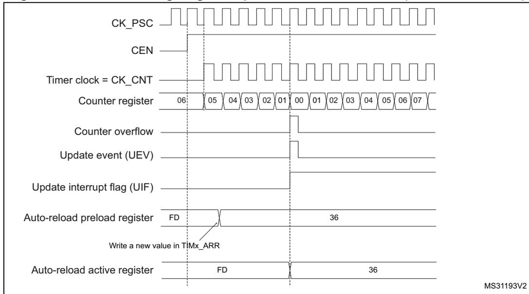
**Figure 208. Counter timing diagram, update event with ARPE=1 (counter overflow)**
