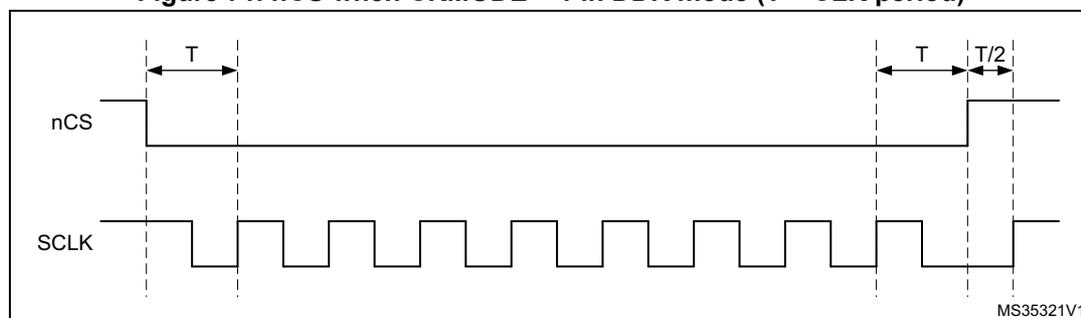
When the FIFO stays full in a read operation or if the FIFO stays empty in a write operation, the operation stalls and CLK stays low until firmware services the FIFO. If an abort occurs when an operation is stalled, nCS rises just after the abort is requested and then CLK rises one half of a CLK cycle later, as shown in *Figure 72*.
