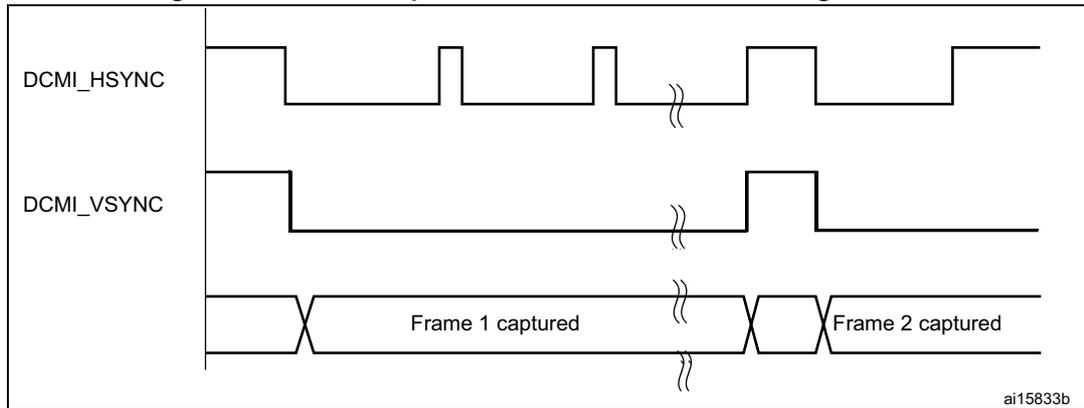
1. Here, the active state of DCMI\_HSYNC and DCMI\_VSYNC is 1.
