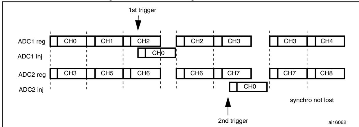
If a trigger occurs during an injected conversion that has interrupted a regular conversion, it is ignored. [Figure 94](#) shows the behavior in this case (2nd trigger is ignored).
