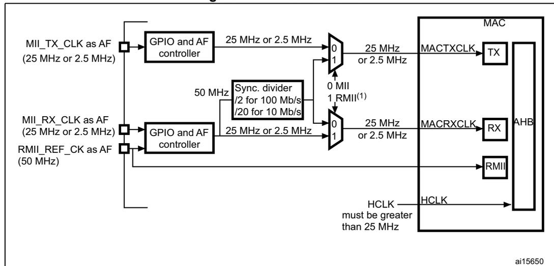
1. The MII/RMII selection is controlled through bit 23, MII\_RMII\_SEL, in the SYSCFG\_PMC register.
