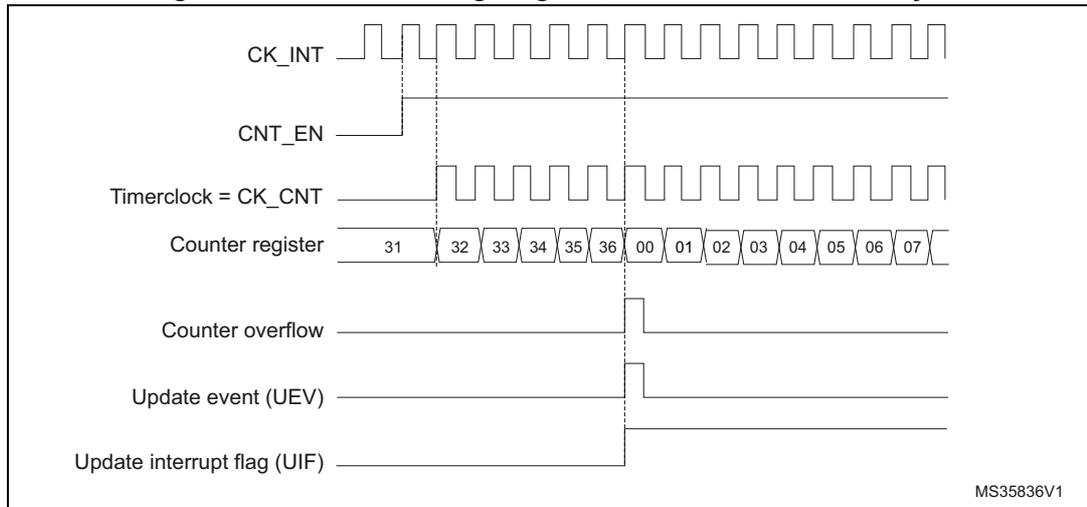
**Figure 241. Counter timing diagram, internal clock divided by 2**
