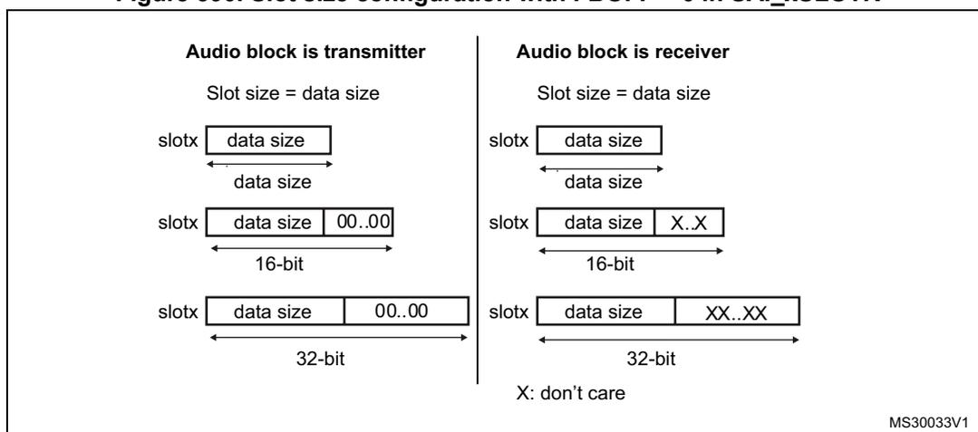
It is possible to choose the position of the first data bit to transfer within the slots. This offset is configured by FBOFF[4:0] bits in the SAI\_xSLOTR register. 0 values will be injected in transmitter mode from the beginning of the slot until this offset position is reached. In reception, the bit in the offset phase is ignored. This feature targets the LSB justified protocol (if the offset is equal to the slot size minus the data size).
