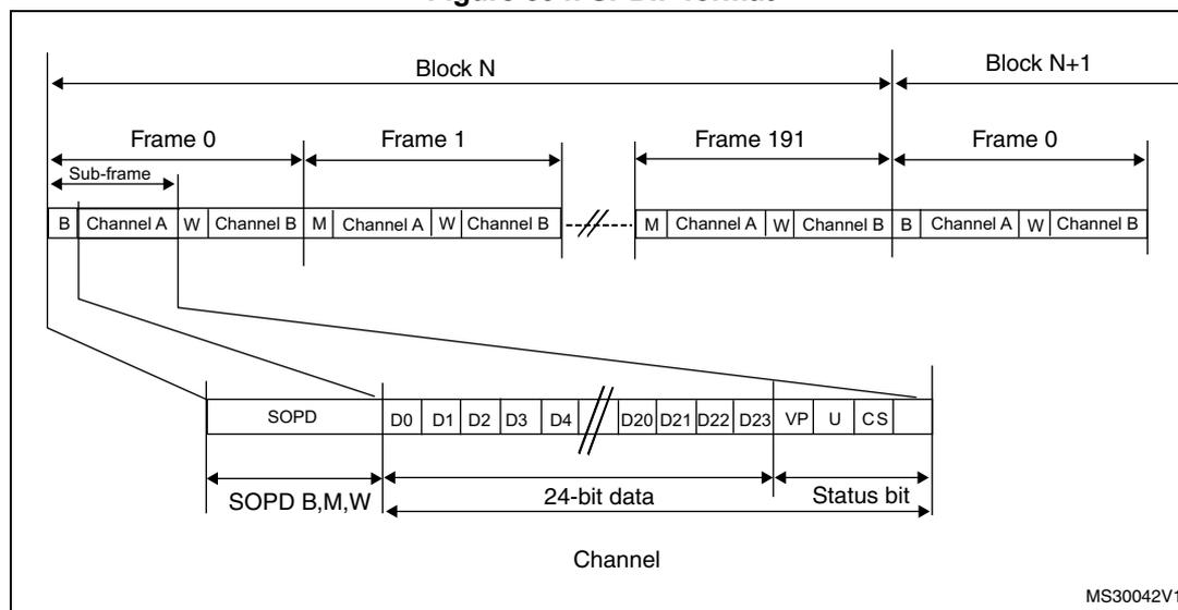
A SPDIF block contains 192 frames. Each frame is composed of two 32-bit sub-frames, generally one for the left channel and one for the right channel. Each sub-frame is composed of a SOPD pattern (4-bit) to specify if the sub-frame is the start of a block (and so is identifying a channel A) or if it is identifying a channel A somewhere in the block, or if it is referring to channel B (see [Table 207](#)). The next 28 bits of channel information are composed of 24 bits data + 4 status bits.
