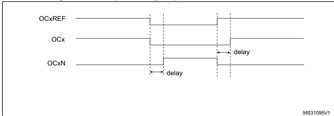
**Figure 224. Dead-time waveforms with delay greater than the negative pulse.**
