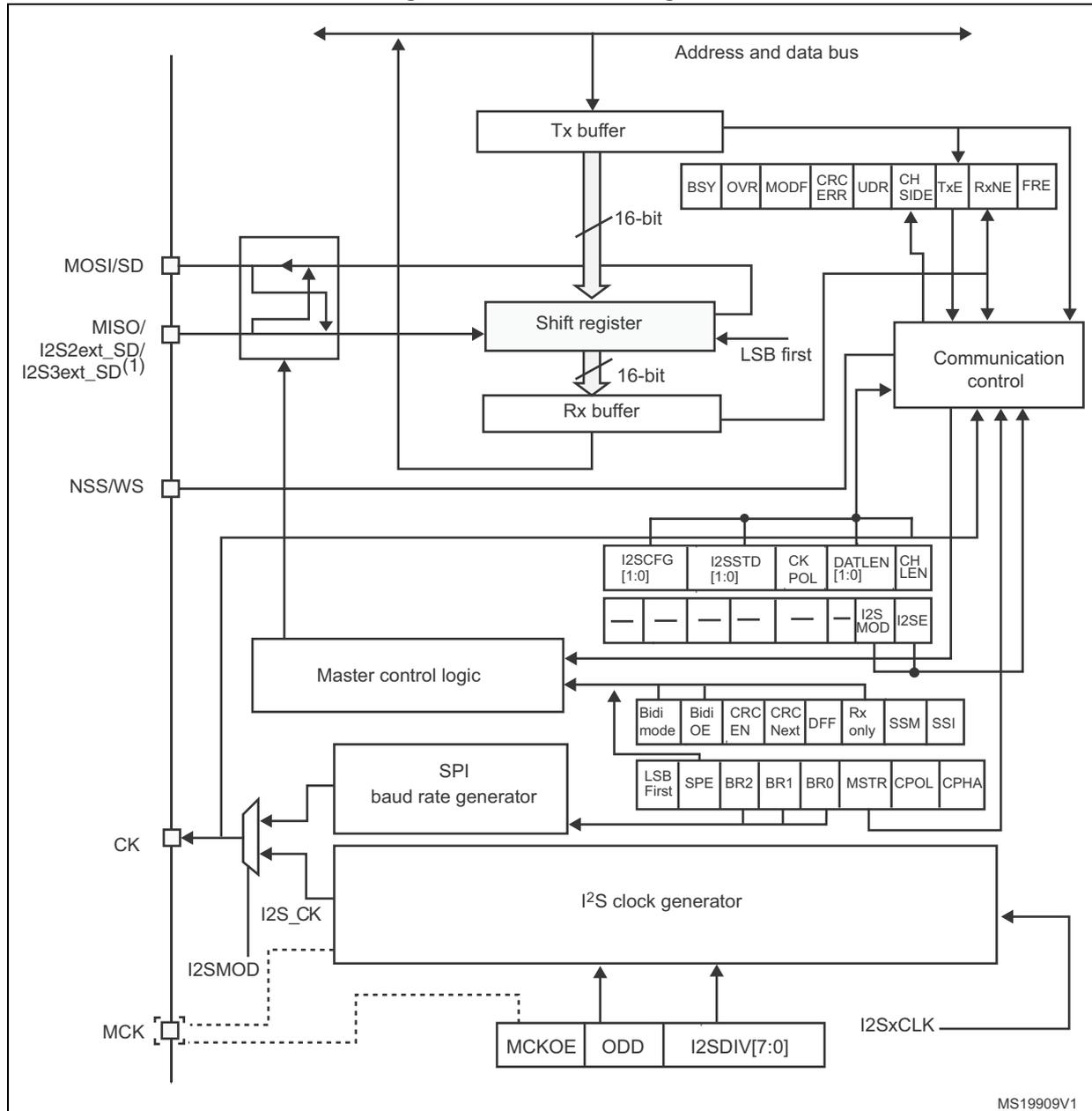
1. I2S2ext\_SD and I2S3ext\_SD are the extended SD pins that control the I2S full-duplex mode.
