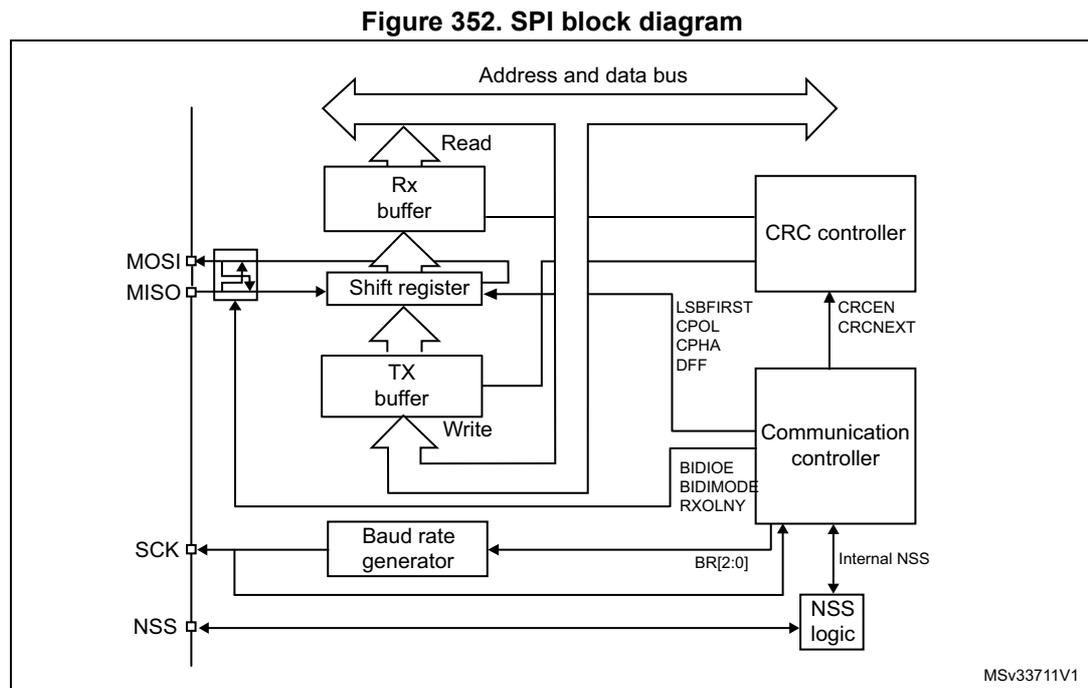
Four I/O pins are dedicated to SPI communication with external devices.
