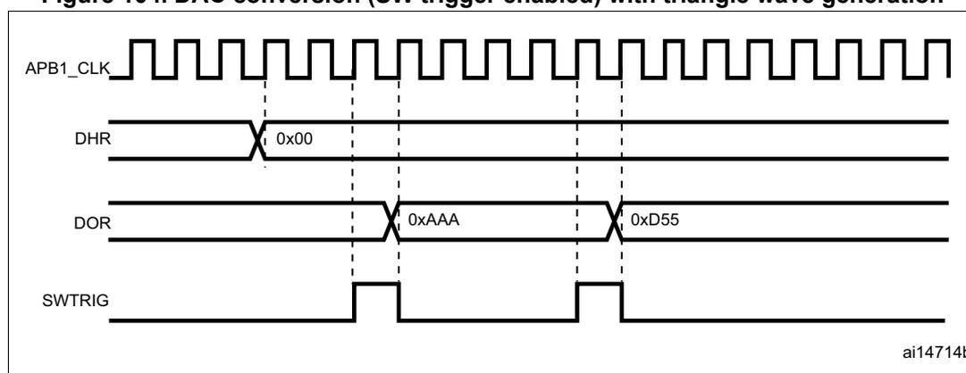
*Note:* The DAC trigger must be enabled for noise generation by setting the TEN<sub>x</sub> bit in the DAC\_CR register.
