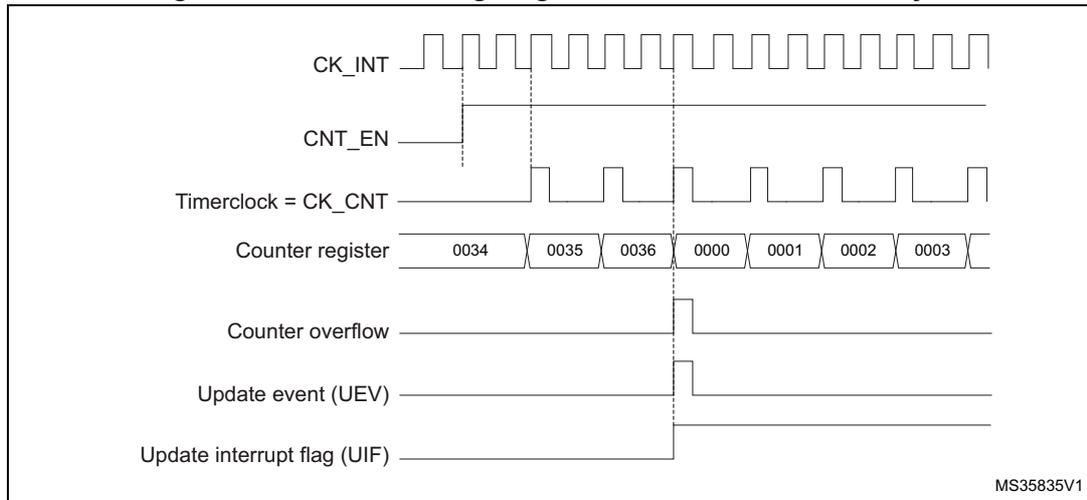
**Figure 311. Counter timing diagram, internal clock divided by 4**
