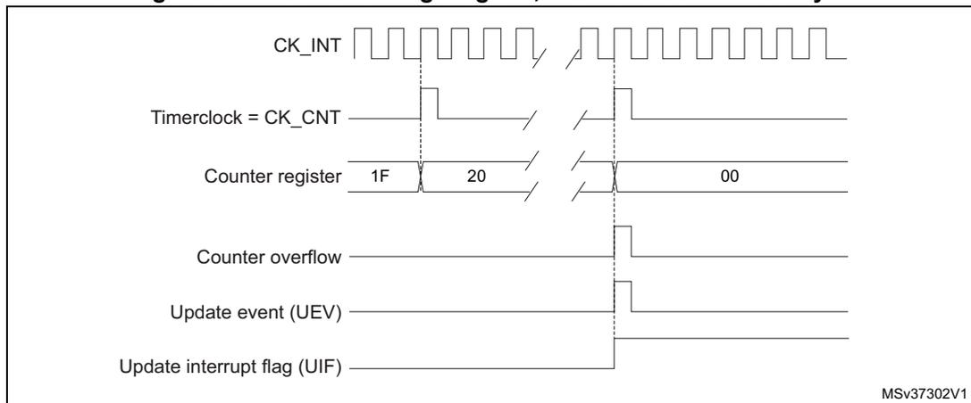
**Figure 313. Counter timing diagram, update event when ARPE = 0 (TIMx\_ARR not preloaded)**
