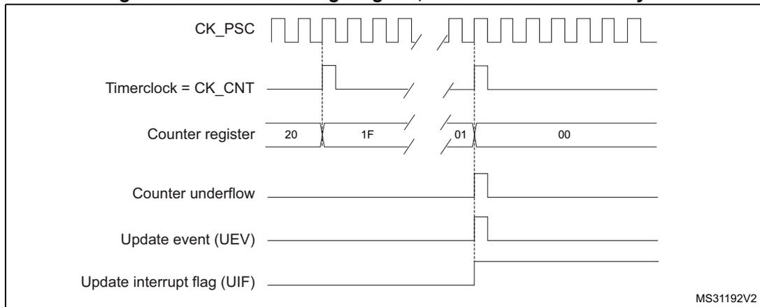
**Figure 207. Counter timing diagram, update event with ARPE=1 (counter underflow)**
