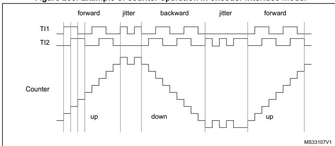
Figure 231 gives an example of counter behavior when TI1FP1 polarity is inverted (same configuration as above except CC1P='1').
