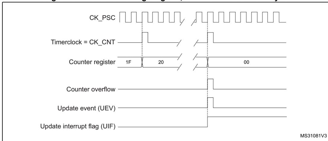
**Figure 196. Counter timing diagram, update event when ARPE=0 (TIMx\_ARR not preloaded)**
