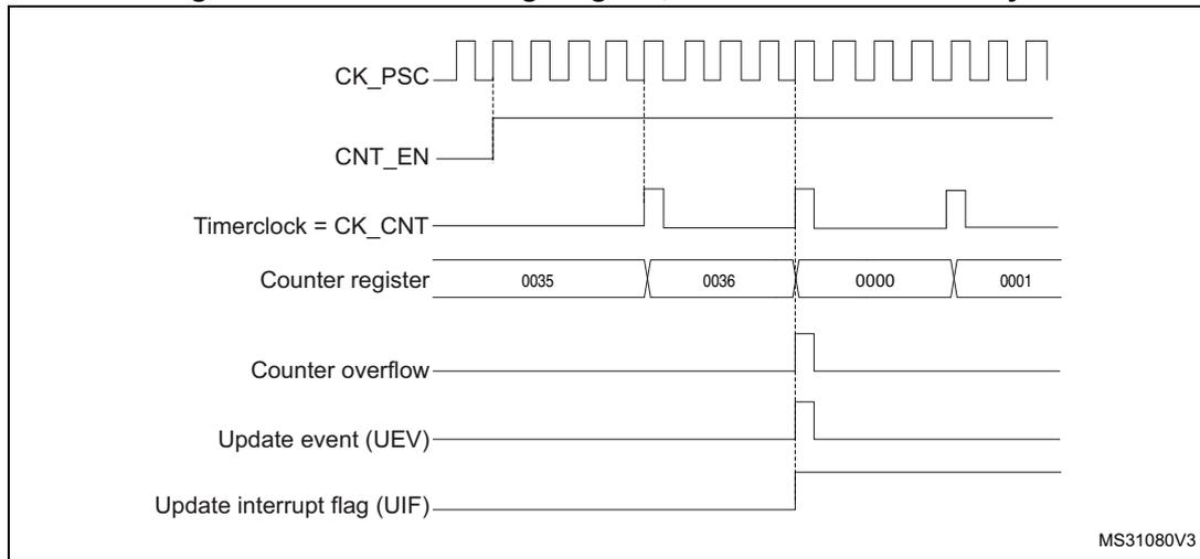
**Figure 195. Counter timing diagram, internal clock divided by N**
