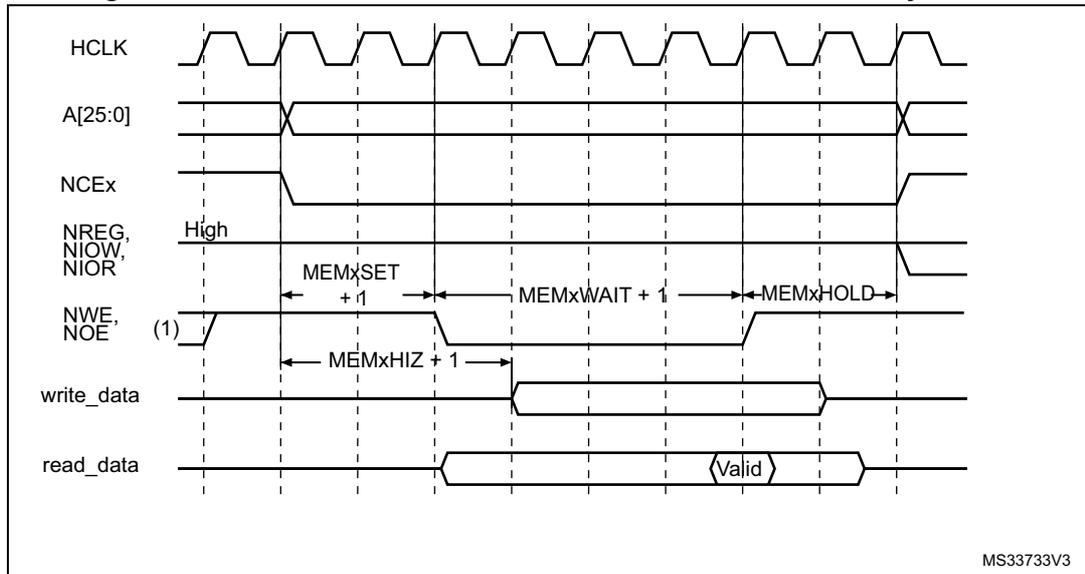
1. NOE remains high (inactive) during write accesses. NWE remains high (inactive) during read accesses.
