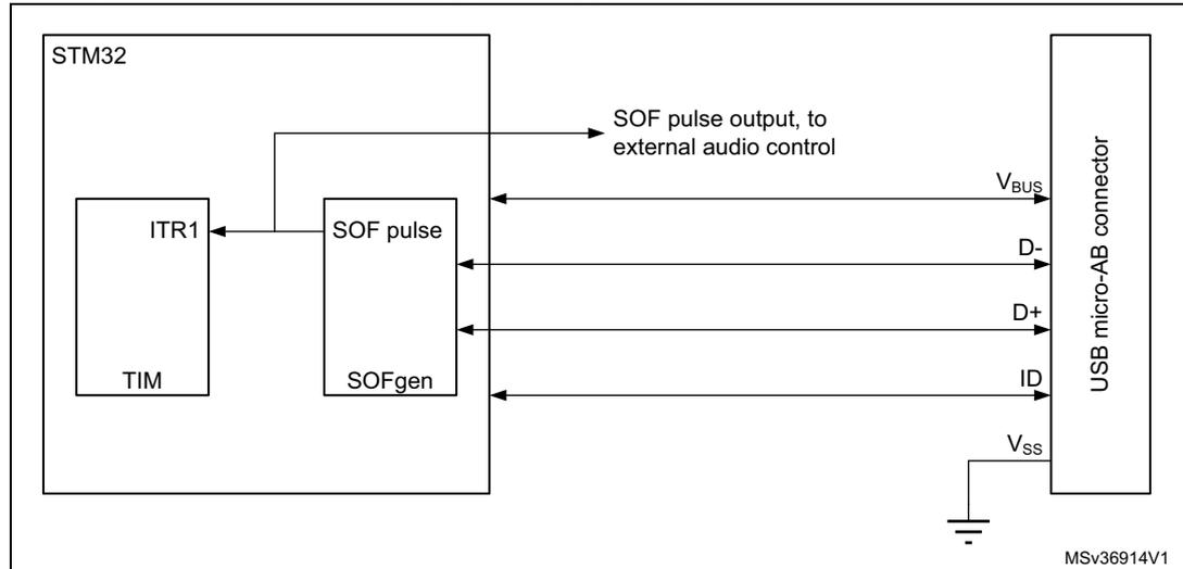
The OTG\_FS/OTG\_HS core provides means to monitor, track and configure SOF framing in the host and peripheral, as well as an SOF pulse output connectivity feature.
