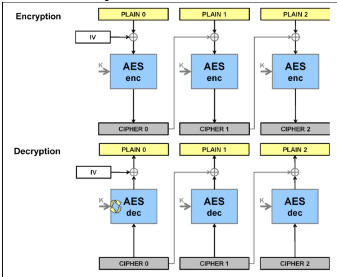
CBC operating mode chains the output of each block with the input of the following block. To make each message unique, an initialization vector is used during the first block processing.
