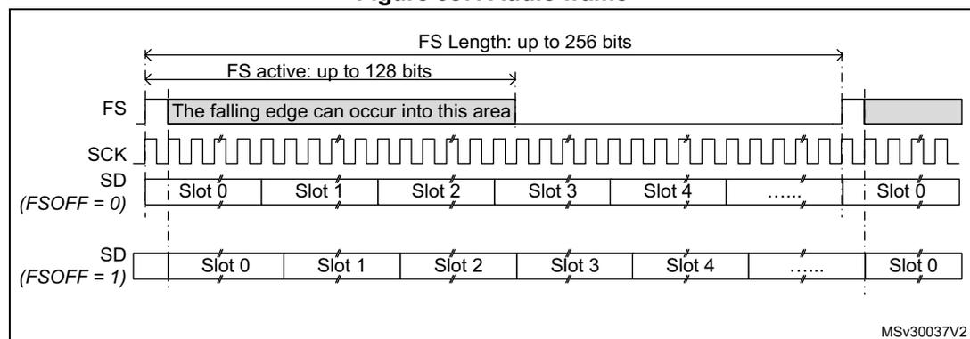
In AC'97 mode or in SPDIF mode (bit PRTCFG[1:0] = 10 or PRTCFG[1:0] = 01 in the SAI\_xCR1 register), the frame synchronization shape is forced to match the AC'97 protocol. The SAI\_xFRCR register value is ignored.
