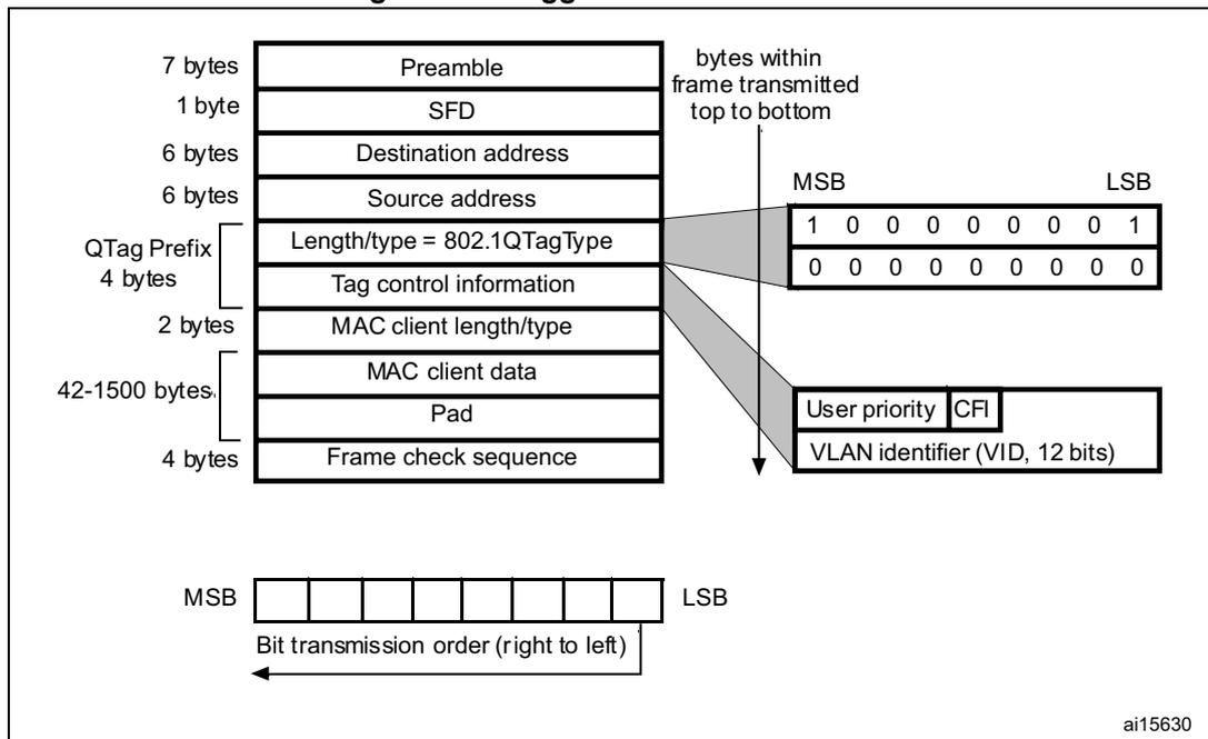
Each byte of the MAC frame, except the FCS field, is transmitted low-order bit first.
