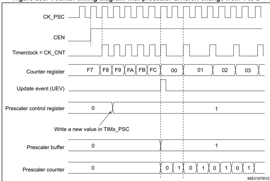
**Figure 286. Counter timing diagram with prescaler division change from 1 to 4**
