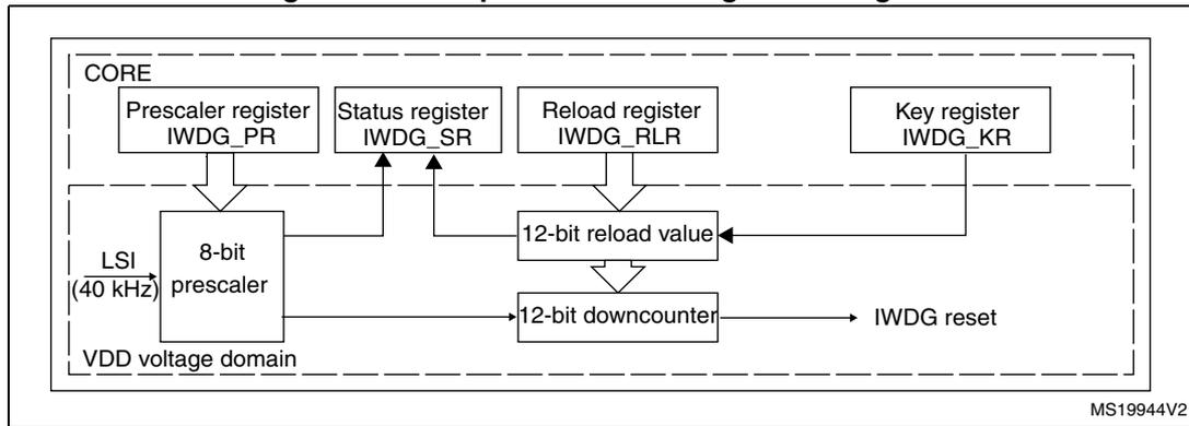
Note: The watchdog function is implemented in the  $V_{DD}$  voltage domain that is still functional in Stop and Standby modes.
