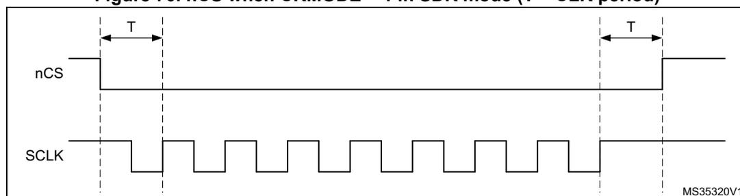
When CKMODE = 1 (“mode3”) and DDRM = 1 (DDR mode), nCS falls one CLK cycle before an operation first rising CLK edge, and nCS rises one CLK cycle after the operation final active rising CLK edge, as shown in *Figure 71*. Because DDR operations must finish with a falling edge, CLK is low when nCS rises, and CLK rises back up one half of a CLK cycle afterwards.
