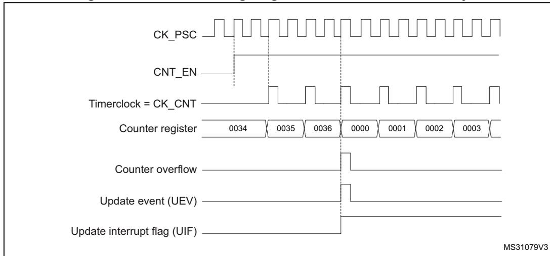
**Figure 194. Counter timing diagram, internal clock divided by 4**
