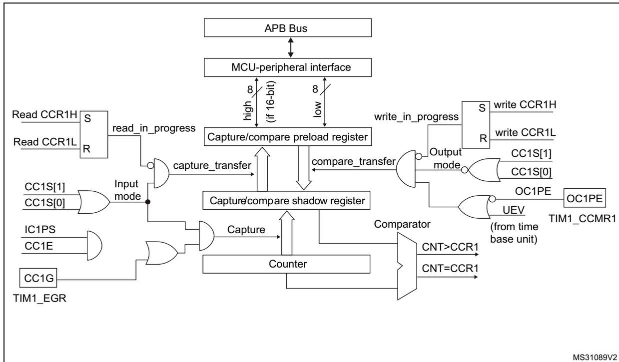
Figure 217. Output stage of capture/compare channel (channels 1 to 3)
