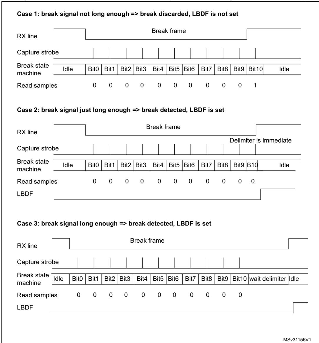
Figure 337. Break detection in LIN mode vs. Framing error detection
