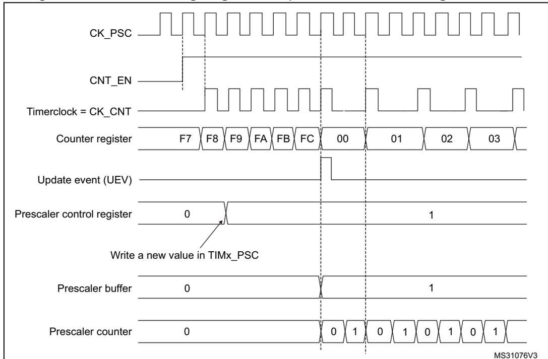
**Figure 308. Counter timing diagram with prescaler division change from 1 to 4**
