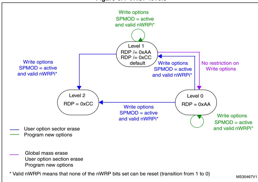
The deactivation of the SPRMOD and/or the unprotection of PCROPed user sectors can only occur when, at the same time, the RDP level changes from 1 to 0. If this condition is not respected, the user option byte modification is cancelled and the write error WRPERR flag is set. The modification of the users option bytes (BOR\_LEV, RST\_STDBY, ..) is allowed since none of the active nWRP<sub>i</sub> bits is reset and SPRMOD is kept active.
