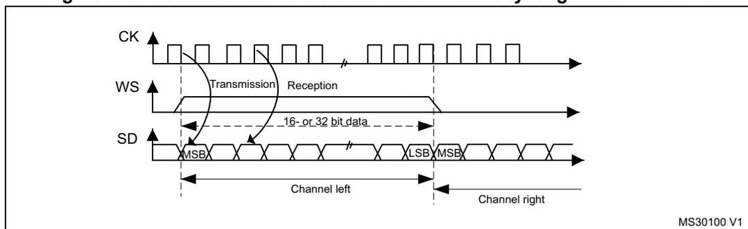
Data are latched on the falling edge of CK (for transmitter) and are read on the rising edge (for the receiver).
