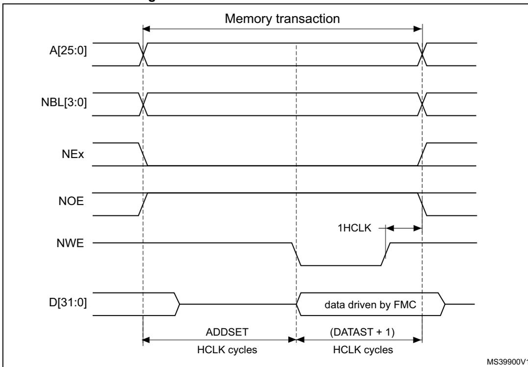
The differences compared with Mode1 are the toggling of NOE and the independent read and write timings.
