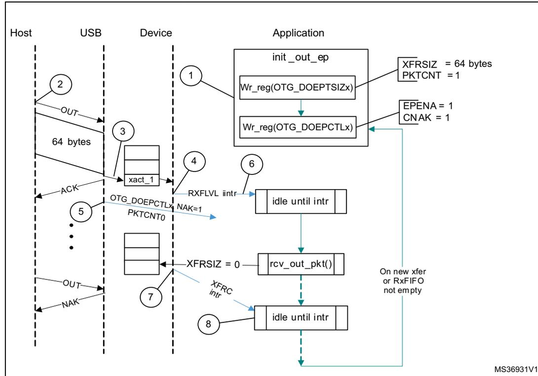
After a SetConfiguration/SetInterface command, the application initializes all OUT endpoints by setting CNAK = 1 and EPENA = 1 (in OTG\_DOEPTLx), and setting a suitable XFRSIZ and PKTCNT in the OTG\_DOEPTSIZx register.
