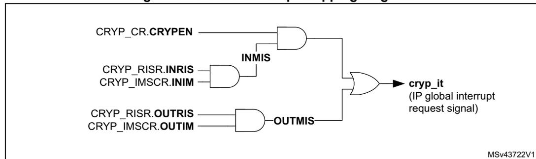
You can enable or disable CRYP interrupt sources individually by changing the mask bits in the CRYP\_IMSCR register. Setting the appropriate mask bit to 1 enables the interrupt.
