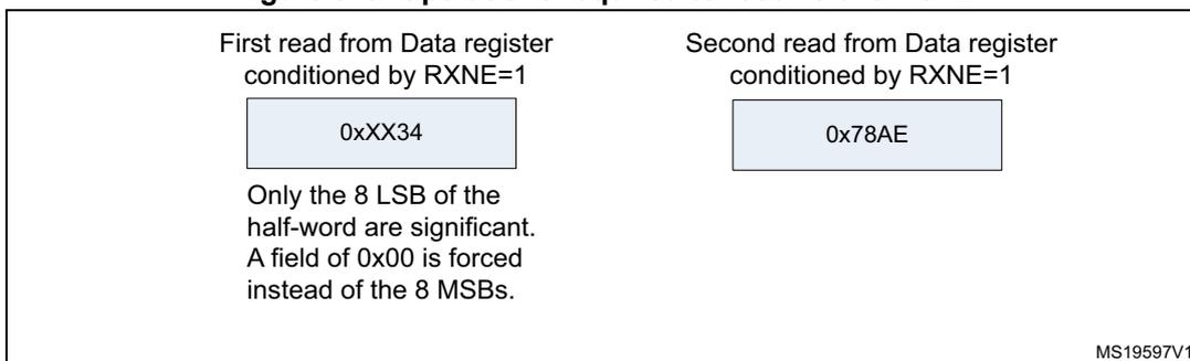
**Figure 380. LSB justified 16-bit extended to 32-bit packet frame with CPOL = 0**
