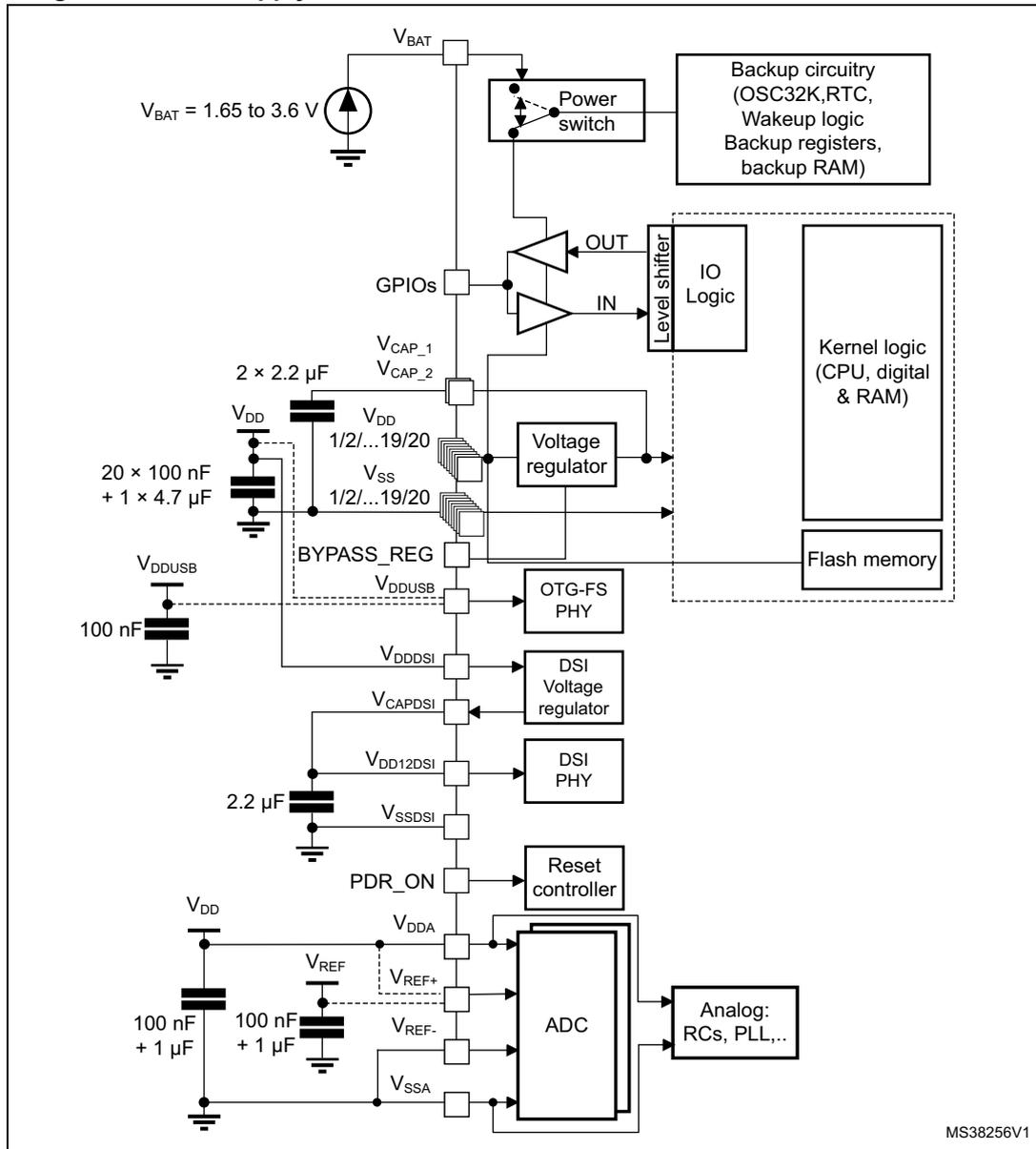
1.  $V_{DDA}$  and  $V_{SSA}$  must be connected to  $V_{DD}$  and  $V_{SS}$ , respectively.
