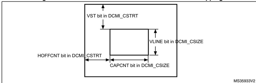
These registers specify the coordinates of the starting point of the capture window as a line number (in the frame, starting from 0) and a number of pixel clocks (on the line, starting from 0), and the size of the window as a line number and a number of pixel clocks. The CAPCNT value can only be a multiple of 4 (two least significant bits are forced to 0) to allow the correct transfer of data through the DMA.
