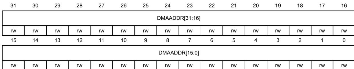
Bits 31:0 **DMAADDR[31:0]**: DMA address
