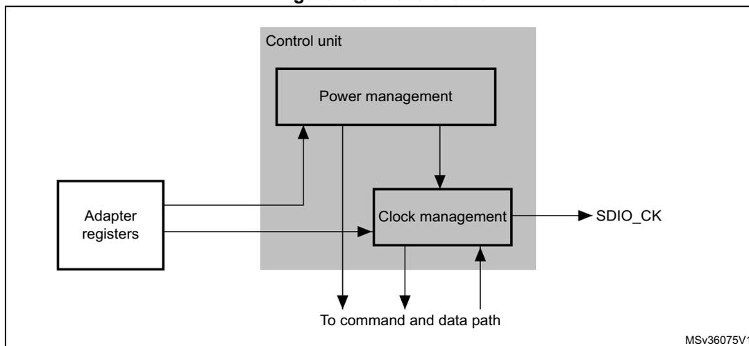
The control unit is illustrated in [Figure 408](#). It consists of a power management subunit and a clock management subunit.
