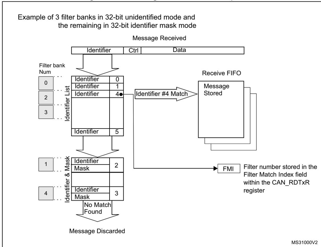
The example above shows the filtering principle of the bxCAN. On reception of a message, the identifier is compared first with the filters configured in identifier list mode. If there is a match, the message is stored in the associated FIFO and the index of the matching filter is stored in the Filter Match Index. As shown in the example, the identifier matches with Identifier #2 thus the message content and FMI 2 is stored in the FIFO.
