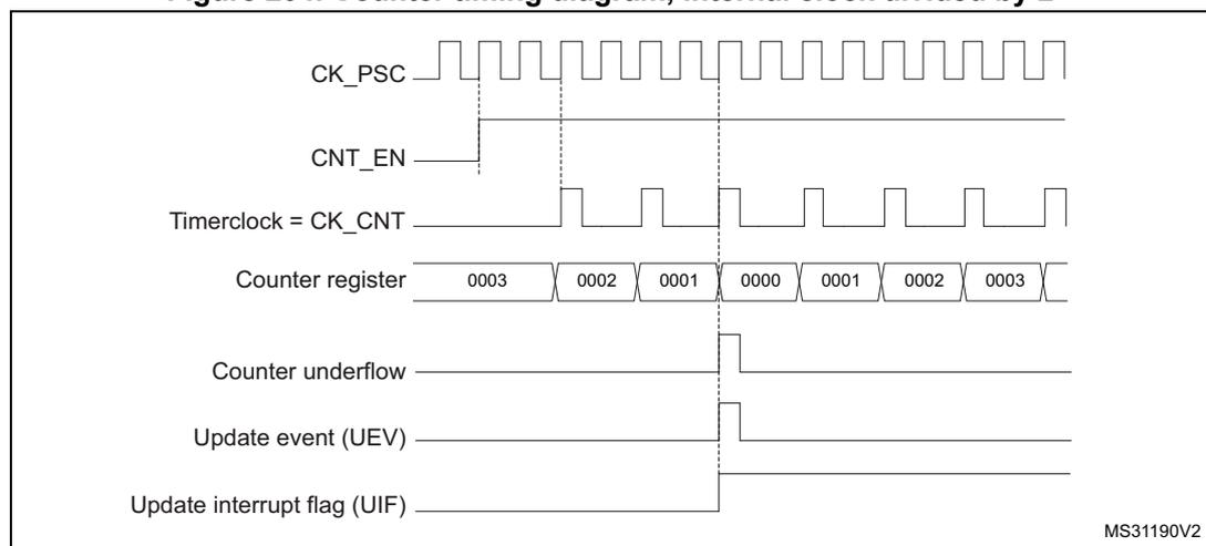
**Figure 205. Counter timing diagram, internal clock divided by 4, TIMx\_ARR=0x36**
