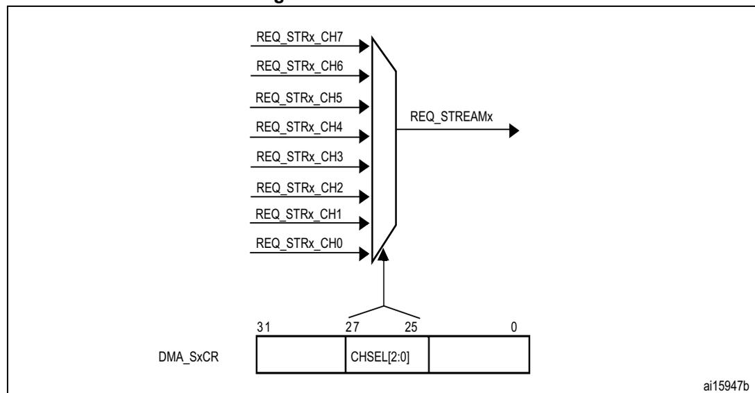
The 8 requests from the peripherals (such as TIM, ADC, SPI, I2C) are independently connected to each channel and their connection depends on the product implementation.
