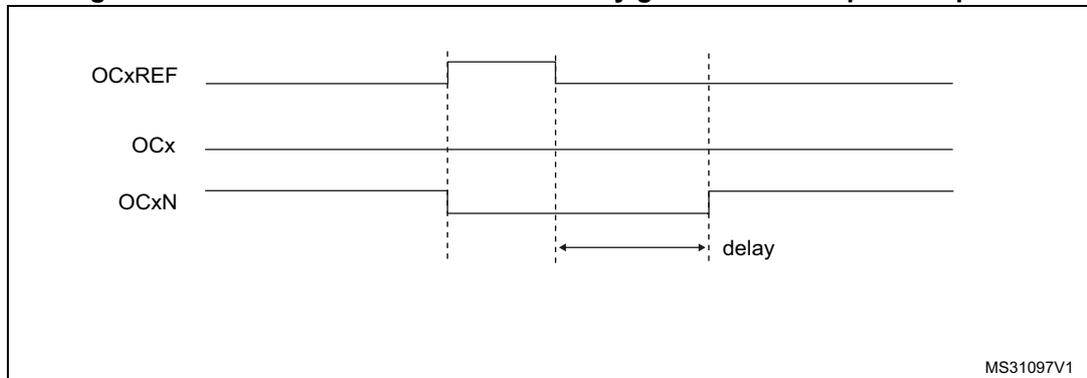
The dead-time delay is the same for each of the channels and is programmable with the DTG bits in the TIMx\_BDTR register. Refer to [Section 22.4.18: TIM1&TIM8 break and dead-time register \(TIMx\\_BDTR\)](#) for delay calculation.
