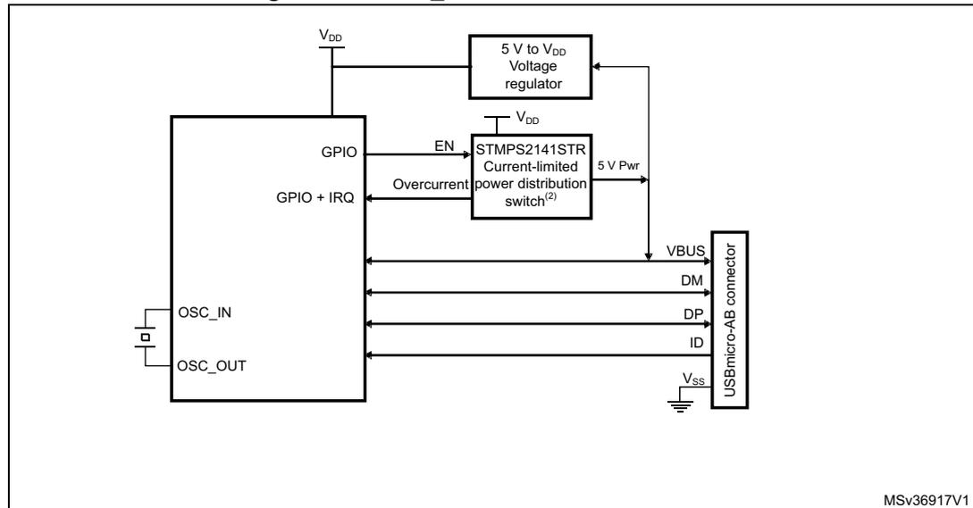
1. External voltage regulator only needed when building a VBUS powered device.
