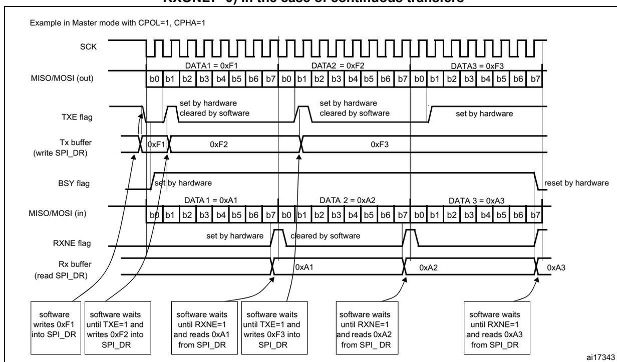
**Figure 361. TXE/RXNE/BSY behavior in slave / full-duplex mode (BIDIMODE=0, RXONLY=0) in the case of continuous transfers**
