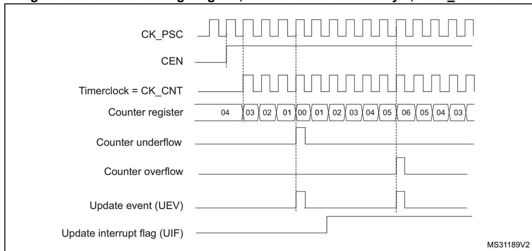
1. Here, center-aligned mode 1 is used (for more details refer to [Section 22.4: TIM1&TIM8 registers](#)).
