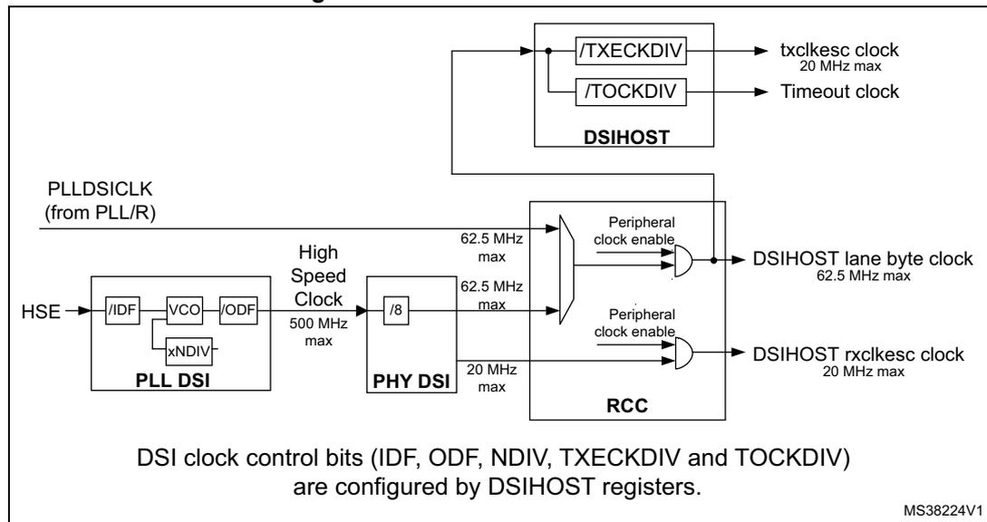
The clock controller provides a high degree of flexibility to the application in the choice of the external crystal or the oscillator to run the core and peripherals at the highest frequency and, guarantee the appropriate frequency for peripherals that need a specific clock like USB OTG FS and HS, I2S, SAI, and SDIO.
