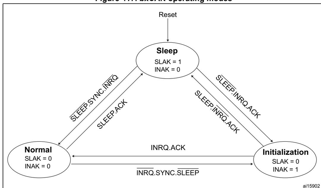
1. ACK = The wait state during which hardware confirms a request by setting the INAK or SLAK bits in the CAN\_MSR register
