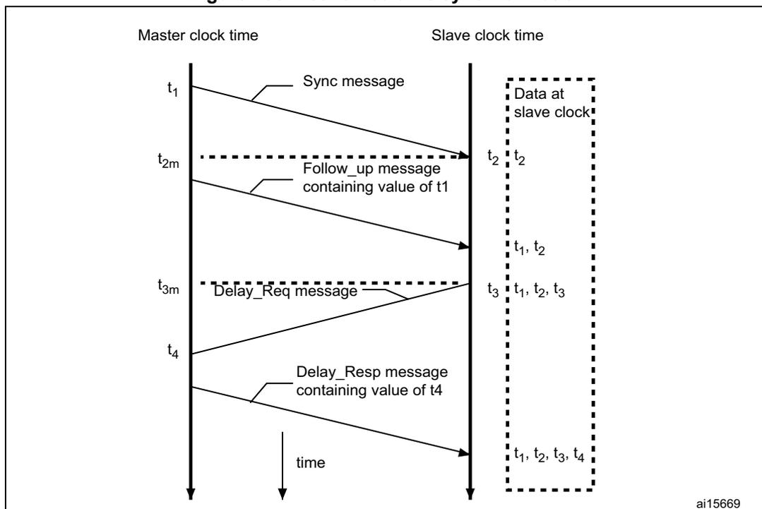
1. The master broadcasts PTP Sync messages to all its nodes. The Sync message contains the master’s reference time information. The time at which this message leaves the master’s system is  $t_1$ . For Ethernet ports, this time has to be captured at the MII.
