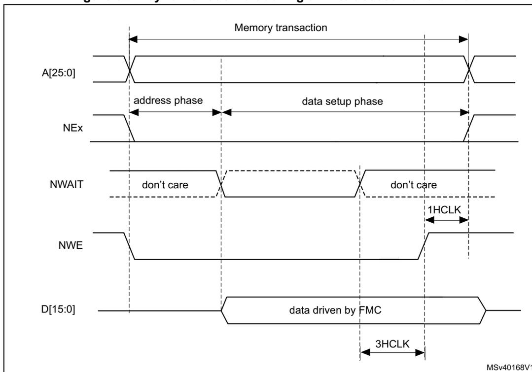
1. NWAIT polarity depends on WAITPOL bit setting in FMC\_BCRx register.
