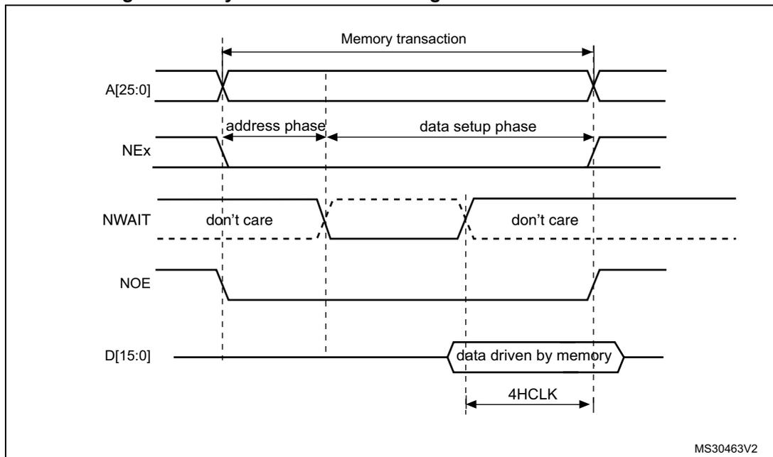
1. NWAIT polarity depends on WAITPOL bit setting in FMC\_BCRx register.
