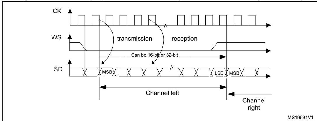
Data are latched on the falling edge of CK (for the transmitter) and are read on the rising edge (for the receiver). The WS signal is also latched on the falling edge of CK.
