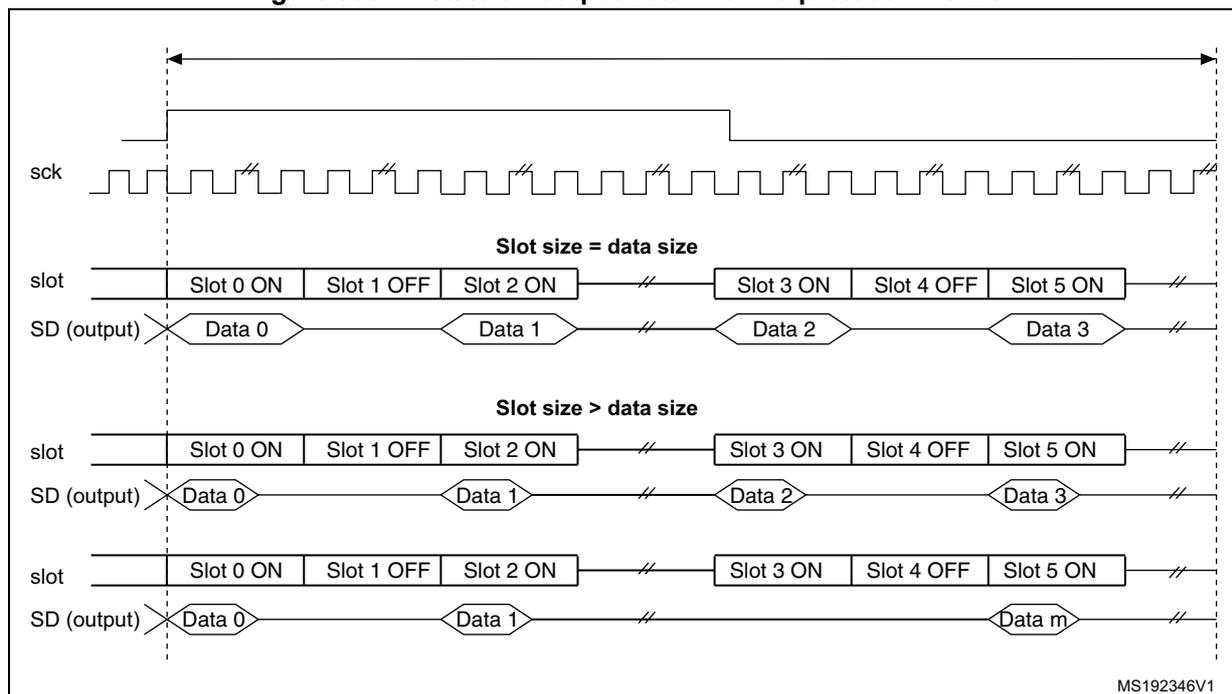
If the TRIS bit in the SAI\_xCR2 register is cleared, all the High impedance states on the SD output line on [Figure 397](#) and [Figure 398](#) are replaced by a drive with a value of 0.
