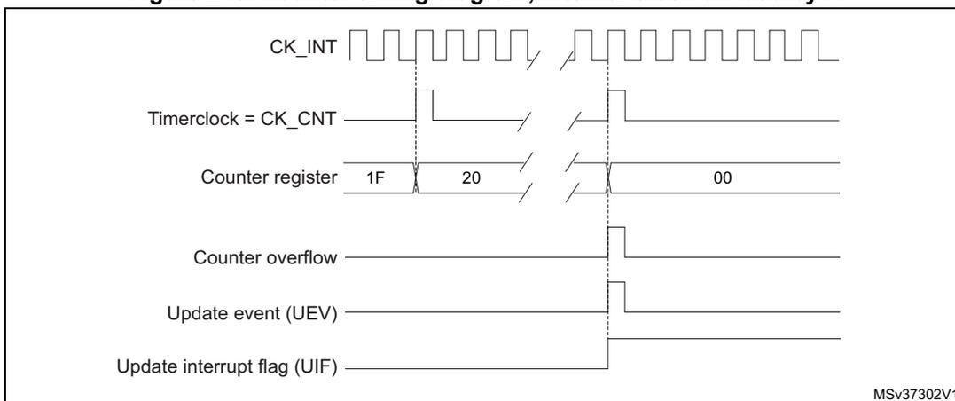
Figure 244. Counter timing diagram, Update event when ARPE=0 (TIMx\_ARR not preloaded)
