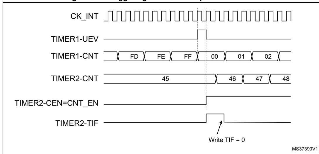
As in the previous example, you can initialize both counters before starting counting. [Figure 281](#) shows the behavior with the same configuration as in [Figure 278](#), but in trigger mode instead of gated mode (SMS=110 in the TIM2\_SMCR register).
