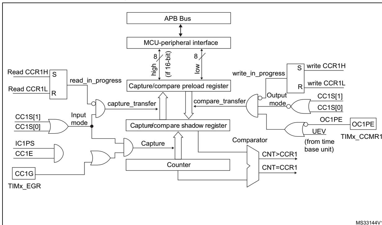
Figure 264. Output stage of capture/compare channel (channel 1)
