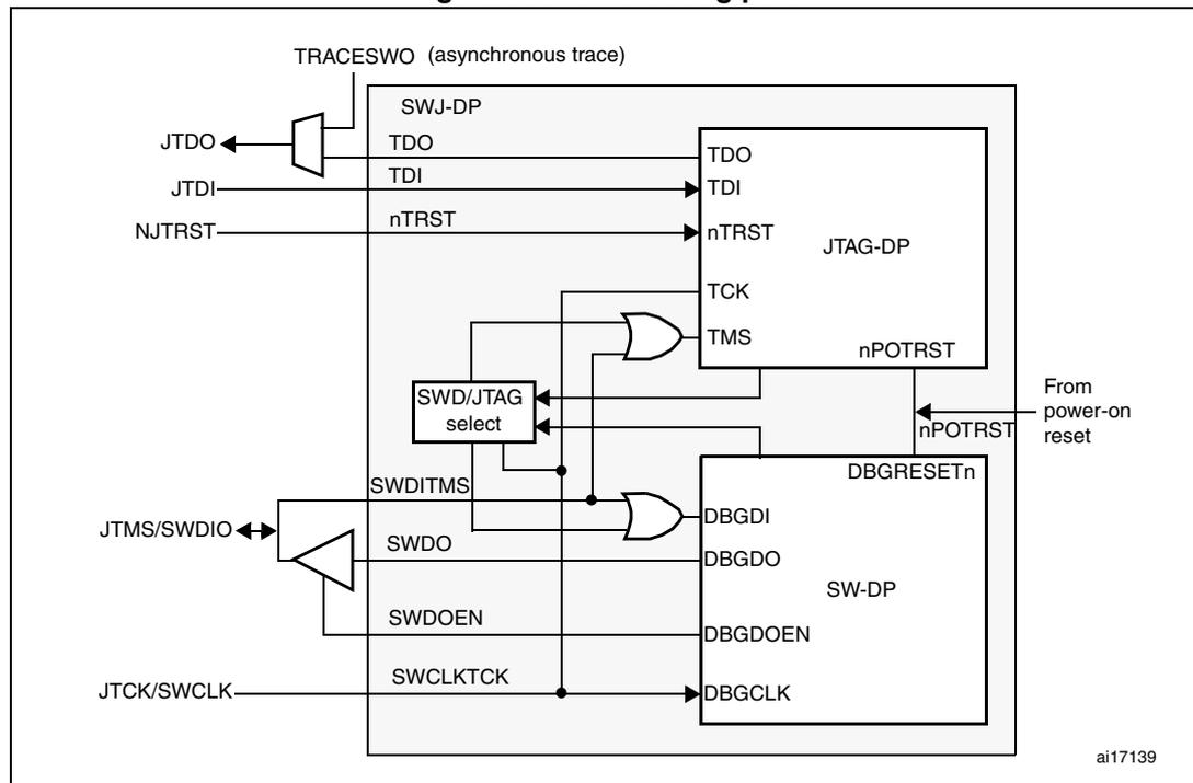
Figure 500 shows that the asynchronous TRACE output (TRACESWO) is multiplexed with TDO. This means that the asynchronous trace can only be used with SW-DP, not JTAG-DP.
