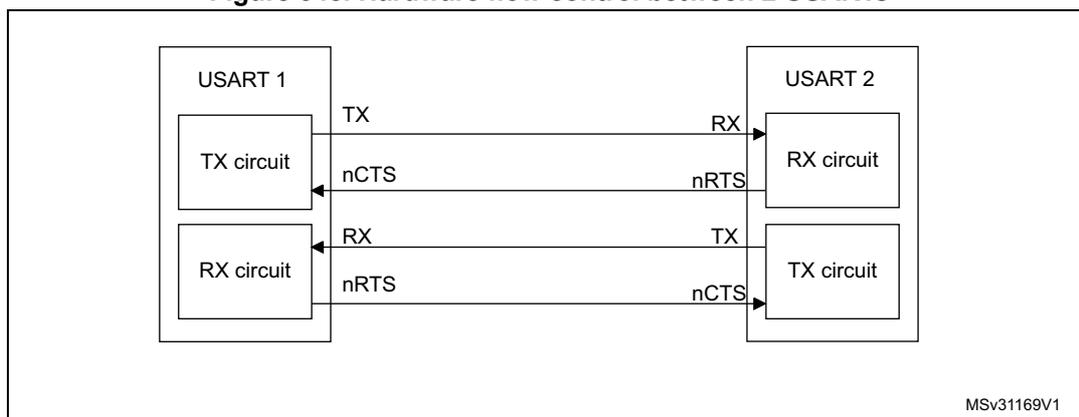
RTS and CTS flow control can be enabled independently by writing respectively RTSE and CTSE bits to 1 (in the USART\_CR3 register).
