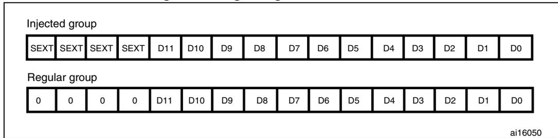
Figure 81. Left alignment of 12-bit data
