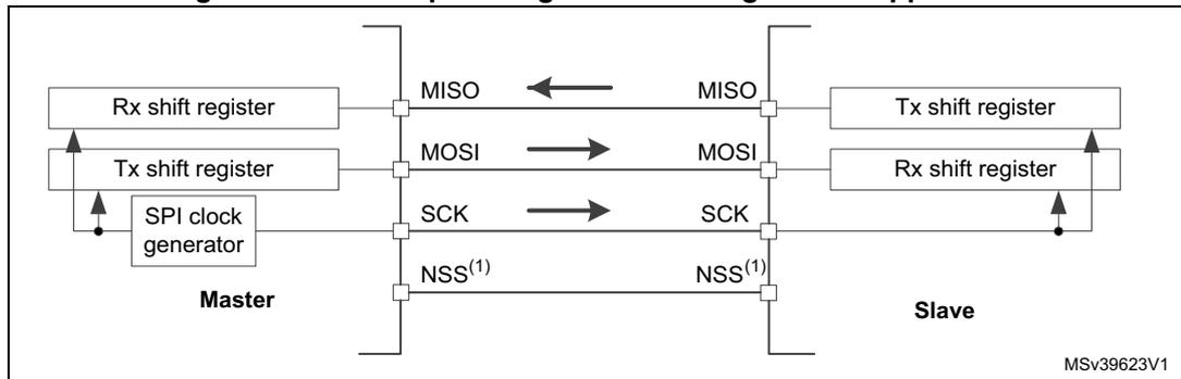
1. The NSS pins can be used to provide a hardware control flow between master and slave. Optionally, the pins can be left unused by the peripheral. Then the flow has to be handled internally for both master and slave. For more details see [Section 31.3.5: Slave select \(NSS\) pin management](#).
