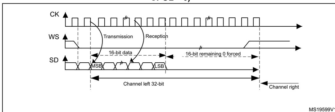
When 16-bit data frame extended to 32-bit channel frame is selected during the I<sup>2</sup>S configuration phase, only one access to the SPIx\_DR register is required. The 16 remaining bits are forced by hardware to 0x0000 to extend the data to 32-bit format.
