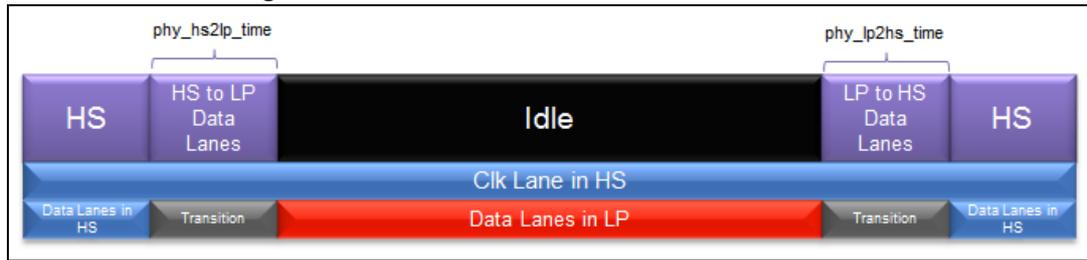
**Figure 144. Clock lane and data lane in LP**
