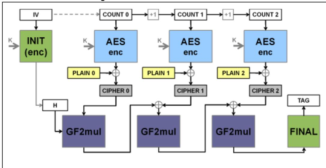
In Galois/Counter mode (GCM), the plaintext message is encrypted, while a message authentication code (MAC) is computed in parallel, thus generating the corresponding ciphertext and its MAC (also known as authentication tag). It is defined in NIST *Special Publication 800-38D, Recommendation for Block Cipher Modes of Operation - Galois/Counter Mode (GCM) and GMAC*.
