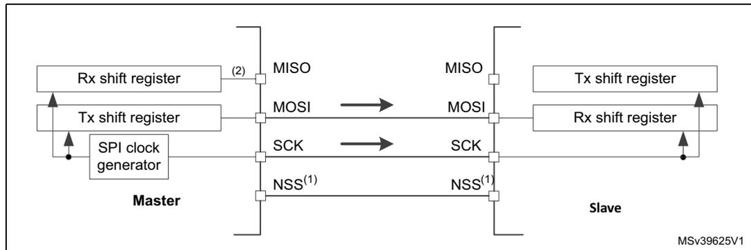
1. The NSS pins can be used to provide a hardware control flow between master and slave. Optionally, the pins can be left unused by the peripheral. Then the flow has to be handled internally for both master and slave. For more details see [Section 31.3.5: Slave select \(NSS\) pin management](#).
