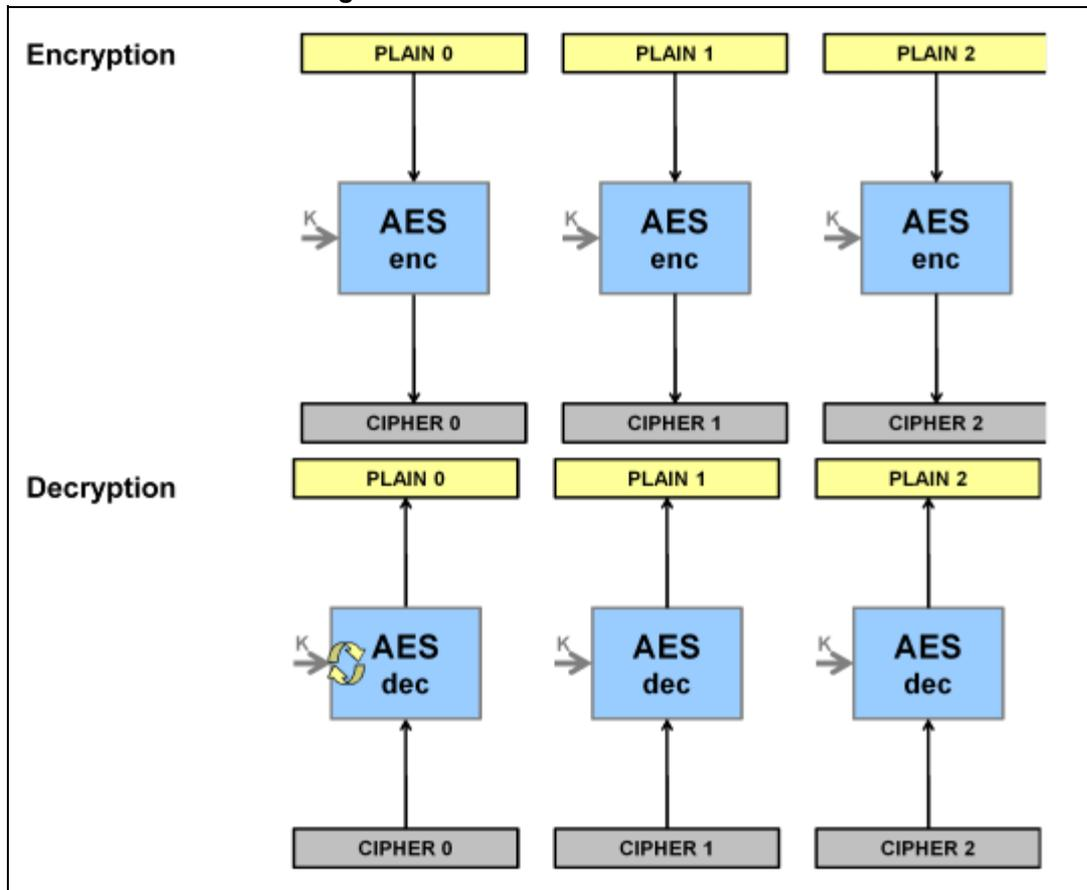
ECB is the simplest operating mode. There are no chaining operations, and no special initialization stage. The message is divided into blocks and each block is encrypted or decrypted separately.
