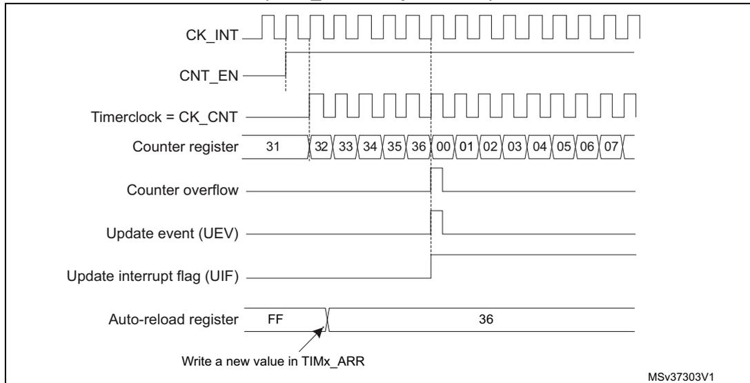
**Figure 314. Counter timing diagram, update event when ARPE=1 (TIMx\_ARR preloaded)**
