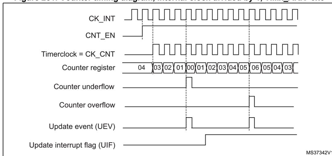
1. Here, center-aligned mode 1 is used (for more details refer to [Section 23.4.1: TIMx control register 1 \(TIMx\\_CR1\)](#) on page 867).
