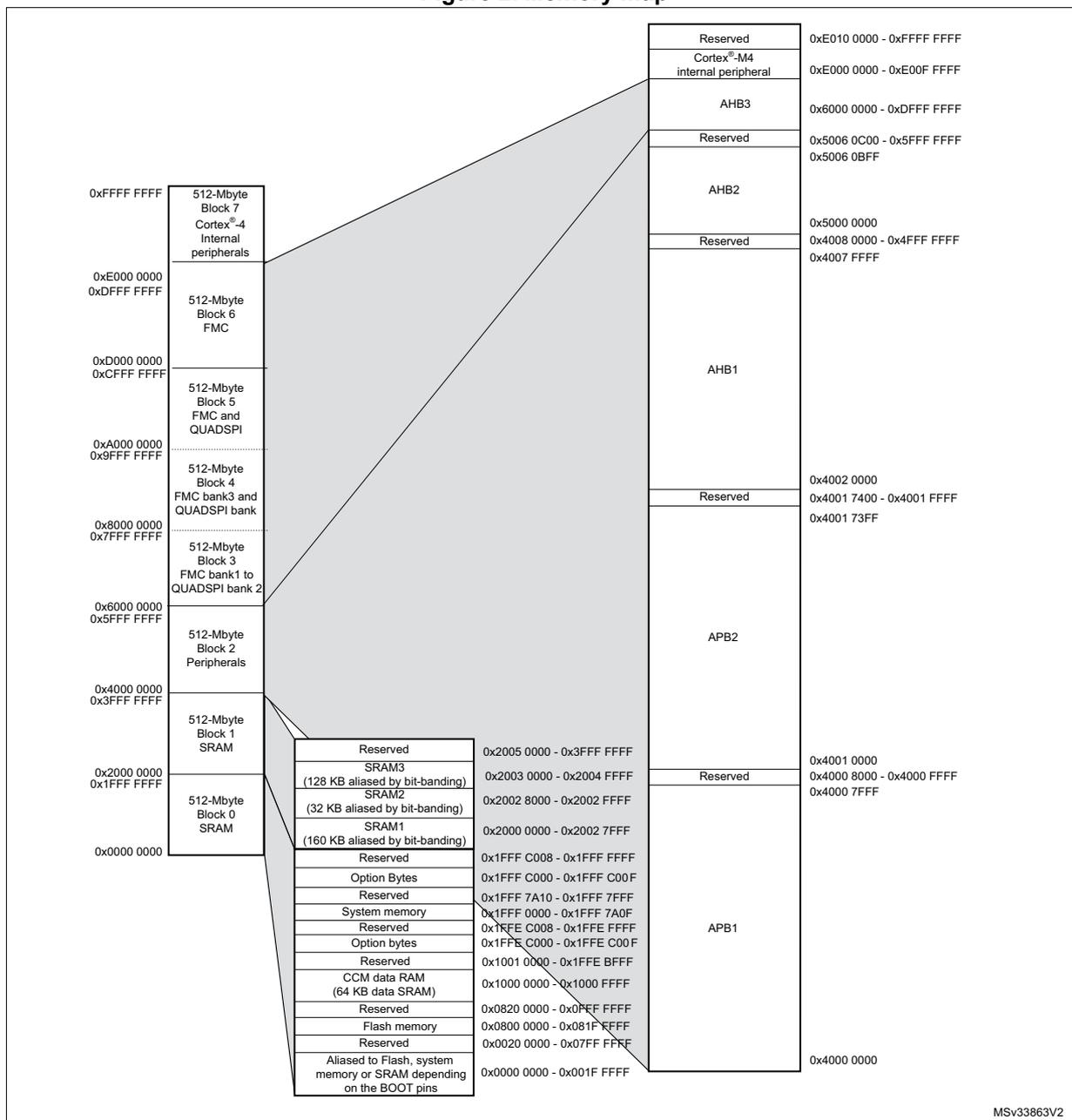
All the memory map areas that are not allocated to on-chip memories and peripherals are considered “Reserved”. For the detailed mapping of available memory and register areas, refer to the following table.
