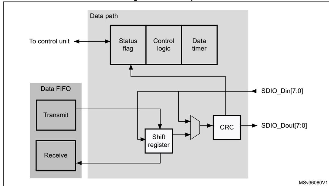
The card databus width can be programmed using the clock control register. If the 4-bit wide bus mode is enabled, data is transferred at four bits per clock cycle over all four data signals (SDIO\_D[3:0]). If the 8-bit wide bus mode is enabled, data is transferred at eight bits per clock cycle over all eight data signals (SDIO\_D[7:0]). If the wide bus mode is not enabled, only one bit per clock cycle is transferred over SDIO\_D0.
