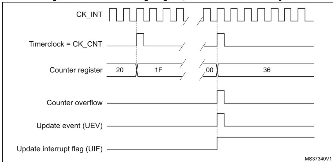
**Figure 250. Counter timing diagram, Update event**
