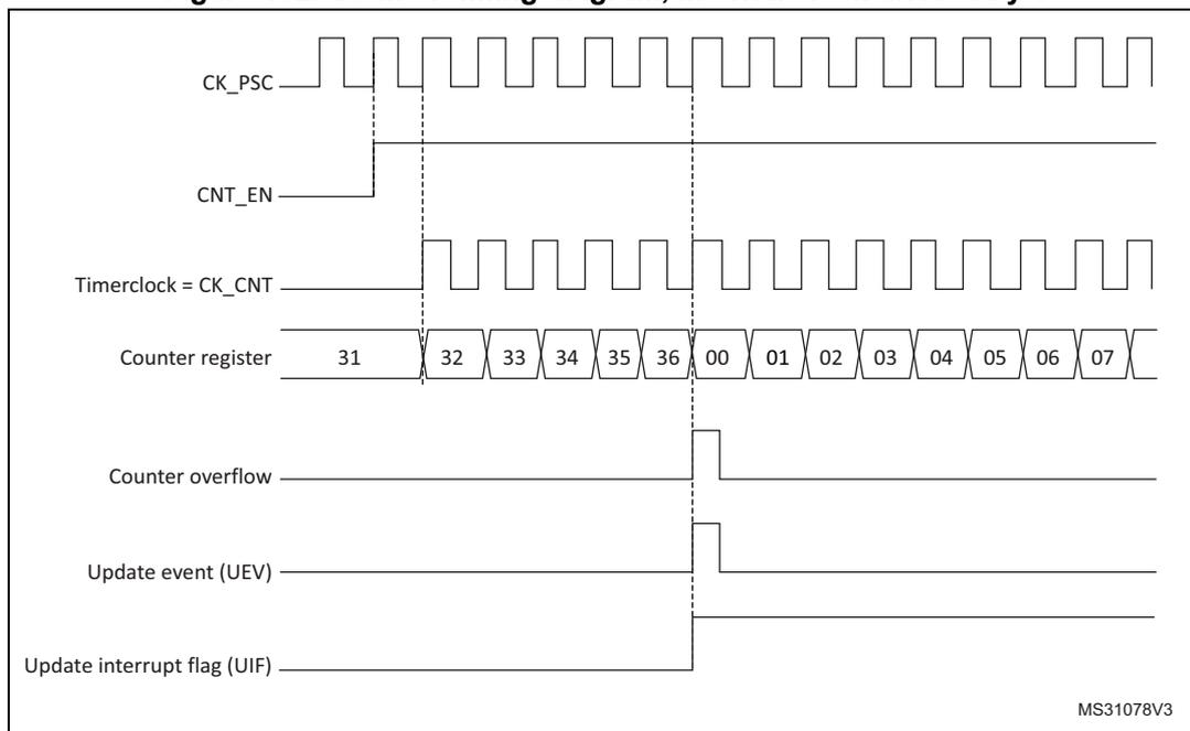
**Figure 193. Counter timing diagram, internal clock divided by 2**
