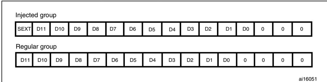
Special case: when left-aligned, the data are aligned on a half-word basis except when the resolution is set to 6-bit. In that case, the data are aligned on a byte basis as shown in [Figure 82](#).
