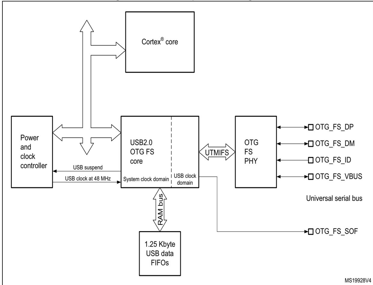
Figure 432. OTG high-speed block diagram
