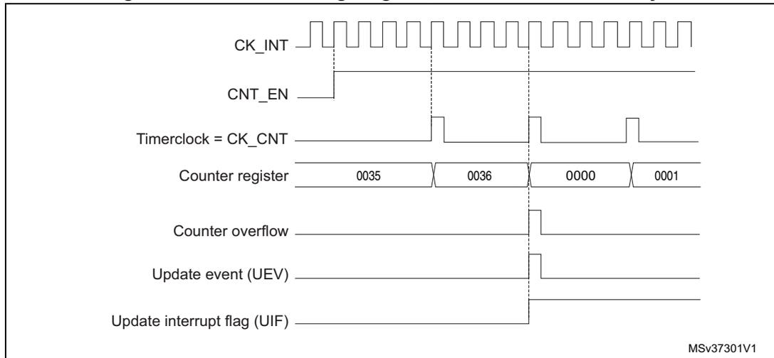
Figure 243. Counter timing diagram, internal clock divided by N
