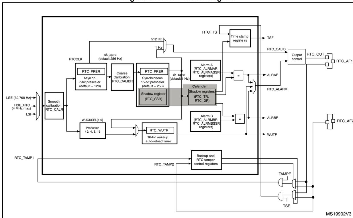
1. On STM32F469xx devices, the RTC\_AF1 and RTC\_AF2 additional function are connected to PC13 and PI8, respectively.
