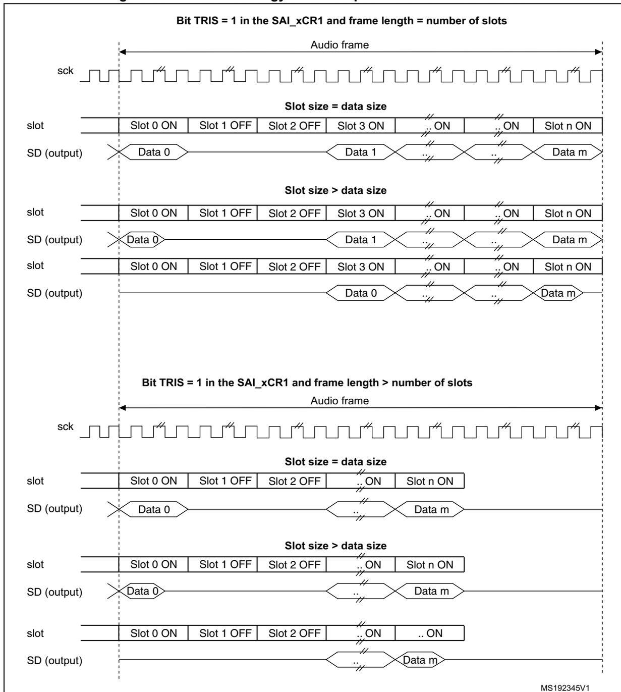
When the selected audio protocol uses the FS signal as a start of frame and a channel side identification (bit FSDEF = 1 in the SAI\_xFRCR register), the tristate mode is managed according to [Figure 398](#) (where bit TRIS in the SAI\_xCR1 register = 1, and FSDEF=1, and half frame length is higher than number of slots/2, and NBSLOT=6).
