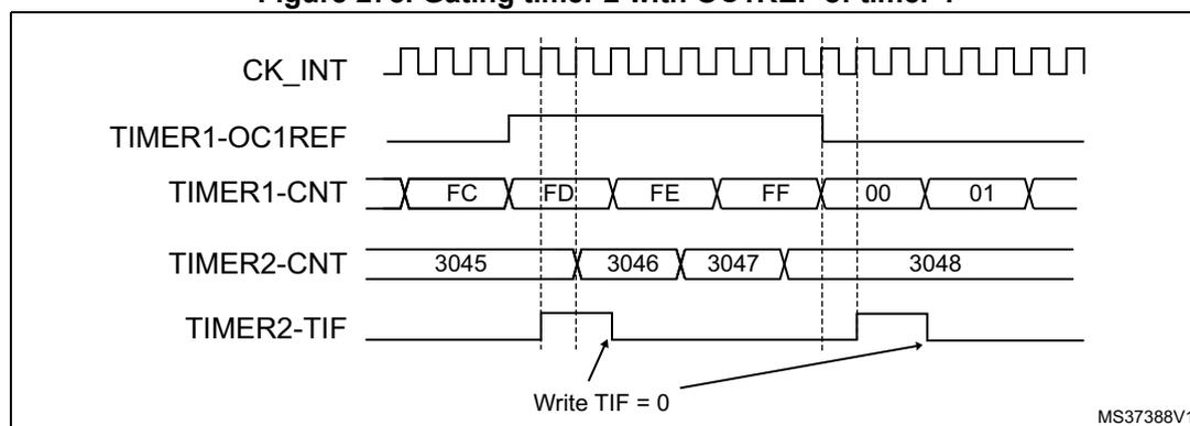
In the example in [Figure 278](#), the Timer 2 counter and prescaler are not initialized before being started. So they start counting from their current value. It is possible to start from a given value by resetting both timers before starting Timer 1. You can then write any value
