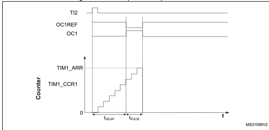
For example you may want to generate a positive pulse on OC1 with a length of  $t_{PULSE}$  and after a delay of  $t_{DELAY}$  as soon as a positive edge is detected on the TI2 input pin.
