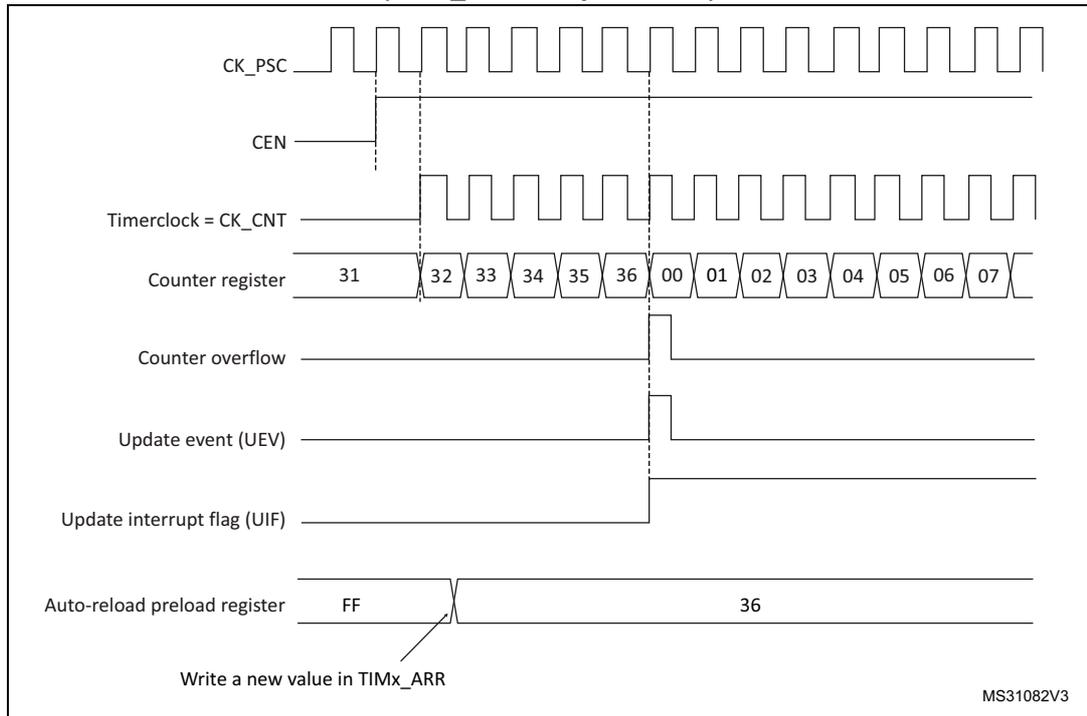
**Figure 197. Counter timing diagram, update event when ARPE=1 (TIMx\_ARR preloaded)**
