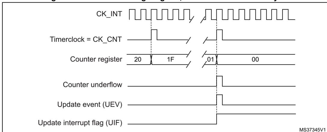
**Figure 255. Counter timing diagram, Update event with ARPE=1 (counter underflow)**
