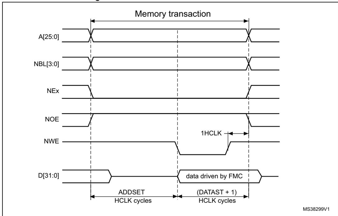
The one HCLK cycle at the end of the write transaction helps guarantee the address and data hold time after the NWE rising edge. Due to the presence of this HCLK cycle, the DATAST value must be greater than zero (DATAST > 0).
