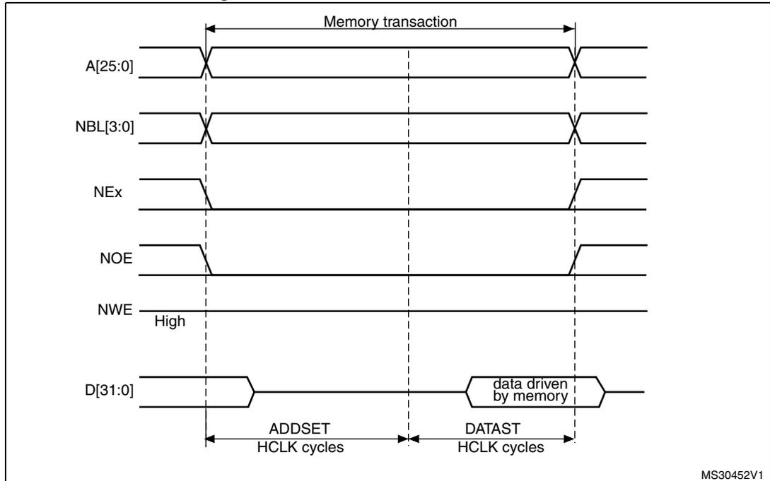
**Figure 39. Mode1 write access waveforms**
