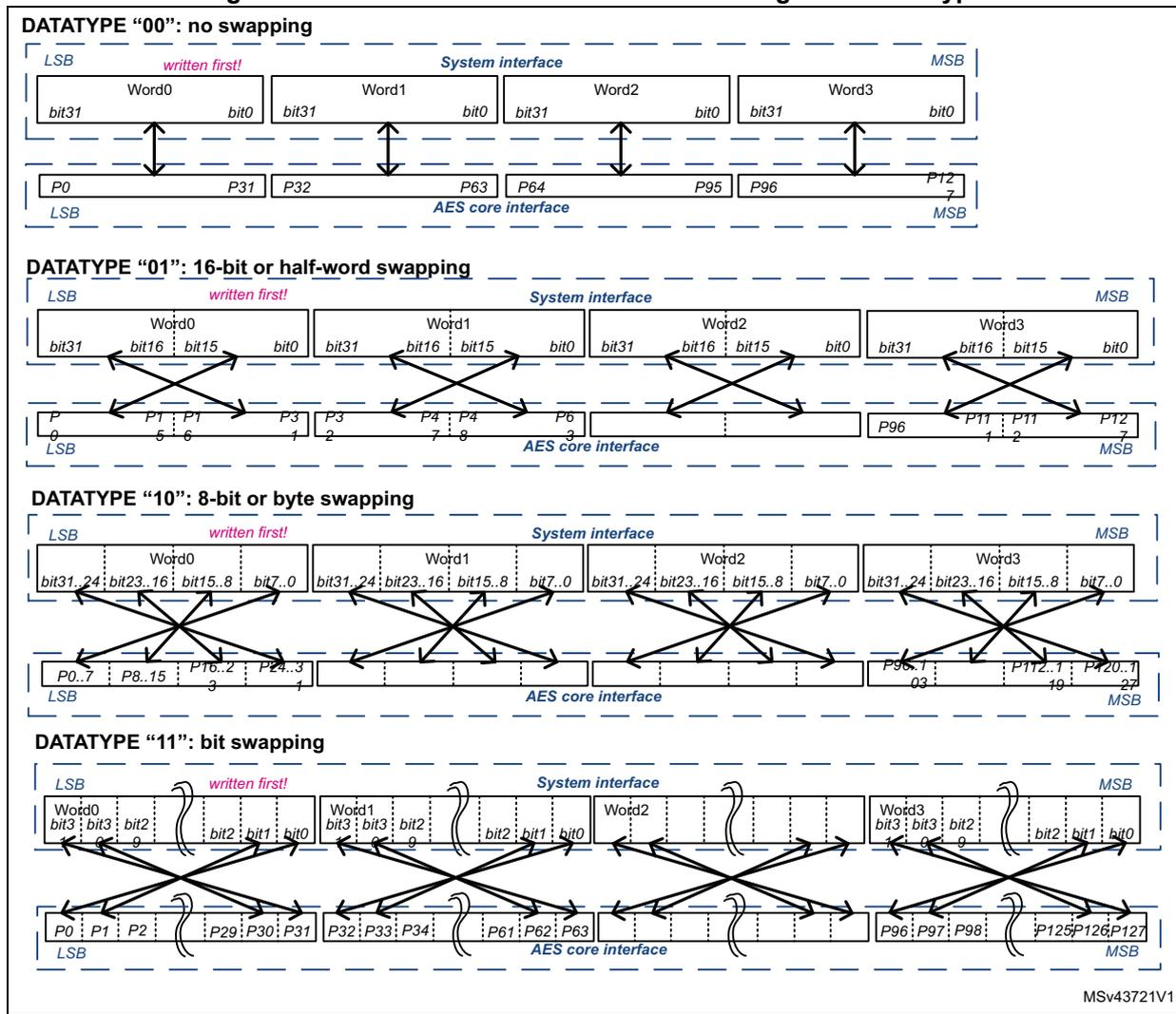
Note: The swapping operation concerns only the CRYP\_DOUT and CRYP\_DIN registers. The CRYP\_KxL/KxR and CRYP\_IVxL/IVxR registers are not sensitive to the swap mode selected. They have a fixed little-endian configuration (refer to Section 20.3.17 and Section 20.3.18).
