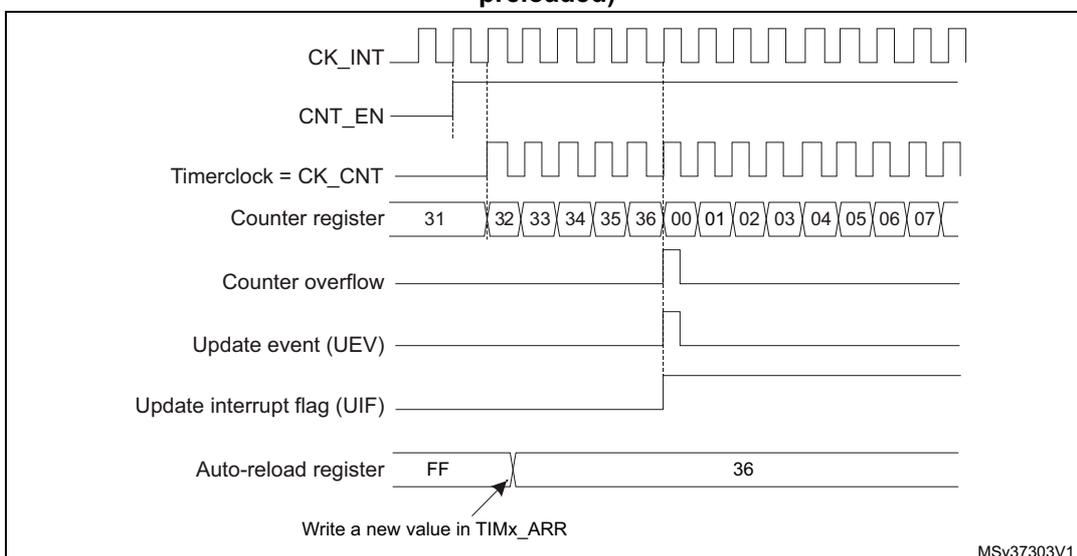
**Figure 245. Counter timing diagram, Update event when ARPE=1 (TIMx\_ARR preloaded)**
