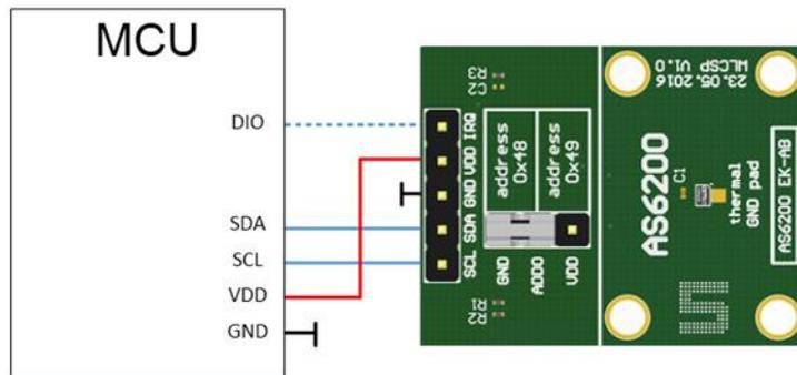
Figure 3: I<sup>2</sup>C connection
