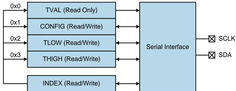
For additional configuration settings the Config register (0x1) has to be addressed. Please refer the data sheet for details.
