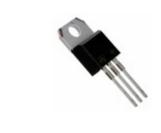
STPS40SM60CT STMicroelectronics DIODE ARRAY SCHOTTKY 60V TO220AB
