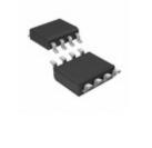
STM706PM6F STMicroelectronics SUPERVISOR 3V WATCHDOG 8SOIC
