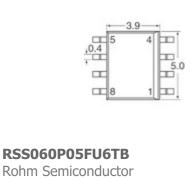
MOSFET P-CH 45V 6A 8-SOIC
