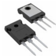
IRFP044NPBF Infineon Technologies MOSFET N-CH 55V 53A TO-247AC
