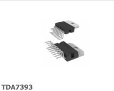
STMicroelectronics IC AMP AUDIO PWR 35W MULTIWATT15
