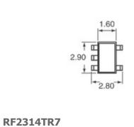
RFMD IC AMP HBT GAAS 2.5GHZ SOT23-5
