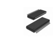
ICS954147BFLFT IDT, Integrated Device Technology Inc IC TIMING CTRL HUB P4 56-SSOP
